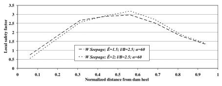
Figure 5. Local sliding safety factor along the dam base for the critical models while seepage is included.
