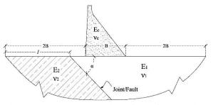
Figure 2. Inhomogeneity of the foundation
