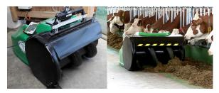
Fig. 1: Target robot platform for feeding with front-facing stereo camera system. Right image: © Wasserbauer
