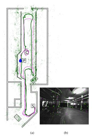
Fig. 3: (a) 3D map from the VSLAM system registered onto the cowshed floor plan; (green) 3D points and trajectory of initial map generation; (purple) trajectory of a subsequent mission. (b) 3D points of map projected onto camera image captured from the blue position *P* in (a). Green dots represent observed 3D points from the initially generated offline map, and purple dots the online generated 3D points.
