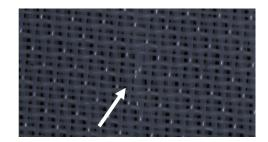
Fig. 1. Two cutouts from the investigated example web patterns with examples of weaving flaws indicated by white arrows. "Pattern 1" (left) and "Pattern 2" (right).
