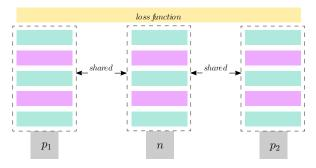
Fig. 5: Triplet architecture
