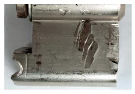
Fig. 1: Snapped lock with multiple toolmarks.
