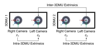
Fig. 2. Illustration of our sensor setup. Please note that cameras are facing the scene, thus left and right are flipped. A detailed description can be found in the text.
