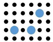
Fig. 3. We use an improved central element [7] for the calibration target, which has the advantage that only three dots in the center have to be visible in order to recognize the pattern, with a high robustness w.r.t. defocusing.
