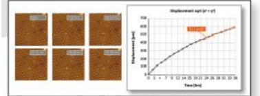
Exceptionally low thermal drift at T=1 K. 36 hours total acqusition time showing a thermal drift stabilising at 11.2 pm/h.
