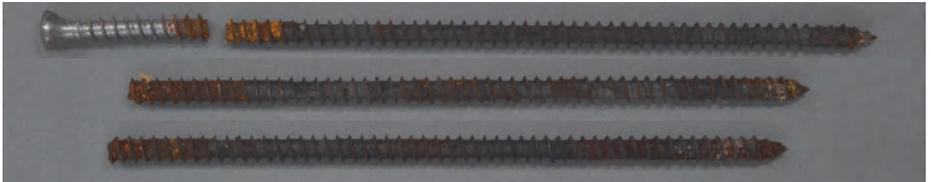
**Figure B.5:** *Macrophotos of A\_s\_I\_08\_240 (zinc-nickel) applied in oak; test campaign I; according to Hauptmann (2016)*
