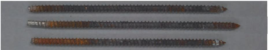
**Figure B.7:** *Macrophotos of A\_s\_IV\_08\_240 (blue chromated) applied in oak; test campaign I; according to Hauptmann (2016)*
