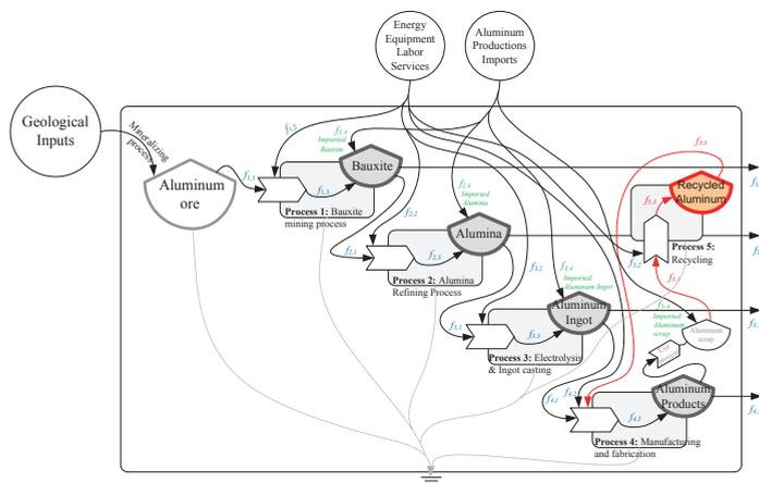
Figure 2.1: The emergy-flow diagram of China's aluminum production system in 2005, showing the main stages of production: bauxite mining (1), alumina refining (2), electrolysis and ingot casting
