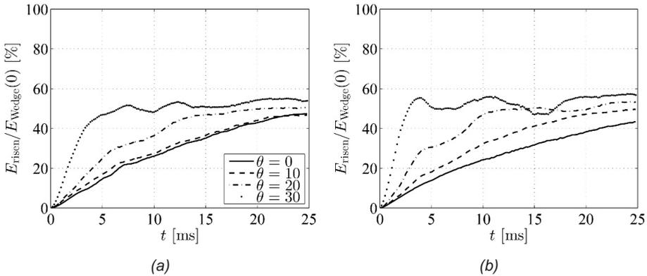
Fig. 4: Average of energy imparted to the risen water  $E_{risen}$  calculated as a percentage of initial wedge energy  $E_{wedge}(0)$  for: (a)  $\alpha = 0^\circ$ , (b)  $\alpha = 10^\circ$ . (Figures adapted from [10])
