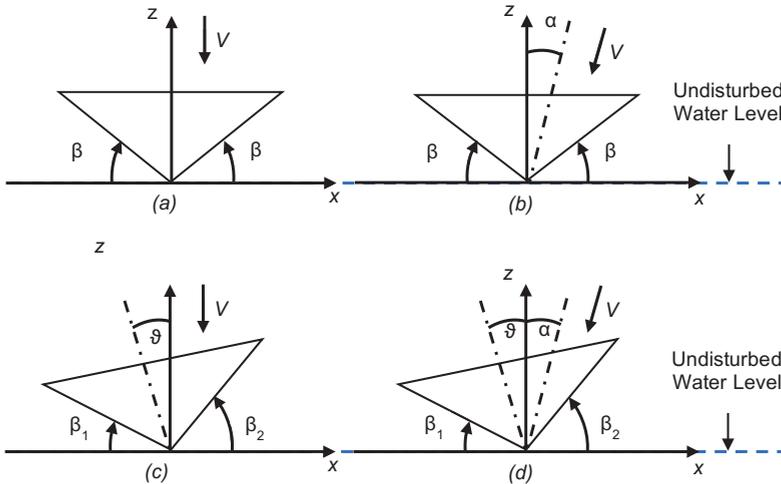
Fig. 2: Experimental Conditions: (a) Vertical Symmetric Impact ( $\alpha = 0$ ;  $\vartheta = 0$ ;  $\beta_1 = \beta_2 = \beta$ ); (b) Oblique Symmetric Impact ( $\alpha > 0$ ;  $\vartheta = 0$ ;  $\beta_1 = \beta_2 = \beta$ ); (c) Asymmetric Impact ( $\alpha = 0$ ;  $\vartheta > 0$ ;  $\beta_1 < \beta_2 > \beta$ ); (d) Oblique Asymmetric Impact ( $\alpha = 0$ ;  $\vartheta = 0$ ;  $\beta_1 = \beta_2 = \beta$ )
