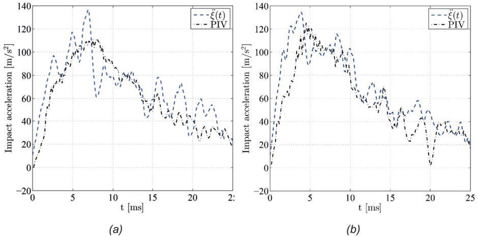
Fig. 3: Average time-histories of impact vertical acceleration acquired through PIV and  $\pm 200g$  piezoelectric accelerometer for: (a)  $\alpha = 0^\circ$  and  $\vartheta = 0^\circ$ , (b)  $\alpha = 10^\circ$  and  $\vartheta = 10^\circ$ .
