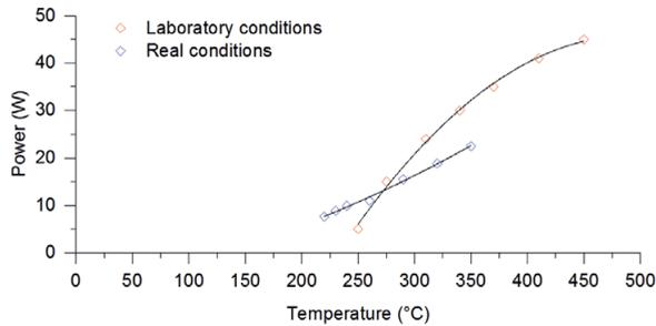
Figure 5: The comparison of TEG No. 1 operating parameters in actual and laboratory conditions.
