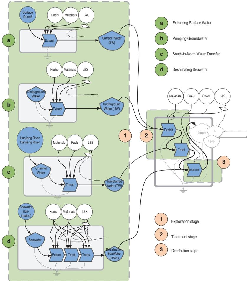
**Fig. 1** Emergy diagram of urban water system in Beijing
