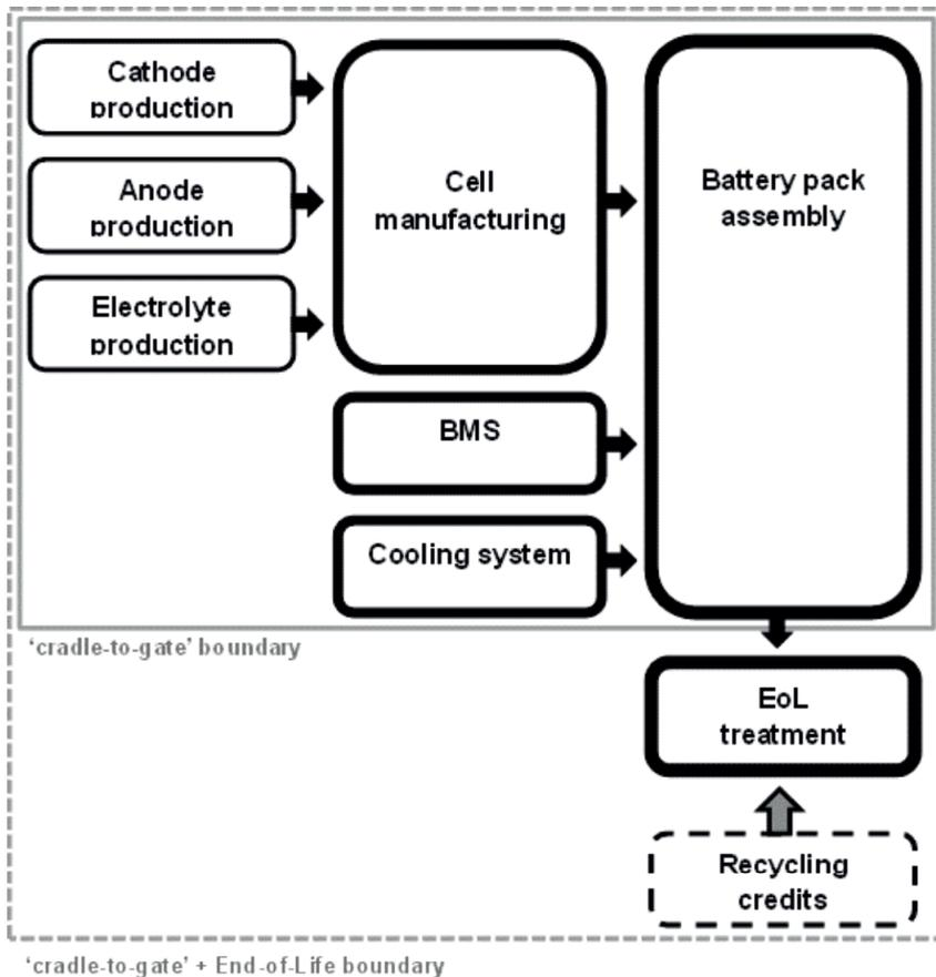
**Figure 1** – Flow diagram of the main steps in the manufacturing of a complete Li-ion battery pack, with indication of optional end-of-life (EoL) treatment and associated recycling credits.
