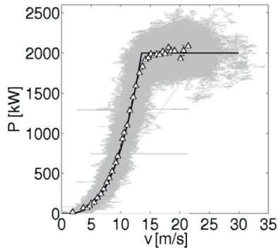
Fig. 7: Power curve for Tjaereborg wind turbine
