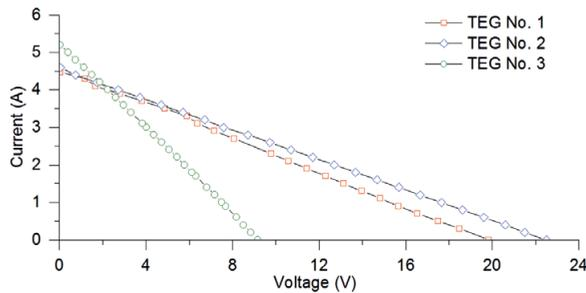
Figure 3: I-V characteristics of the thermoelectric generators.
