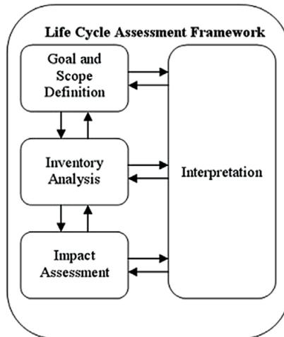
Figure 1. LCA framework
