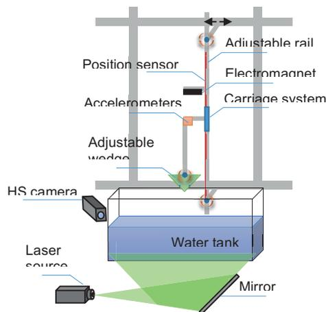
Fig. 1: Simplified sketch of experimental test bench
