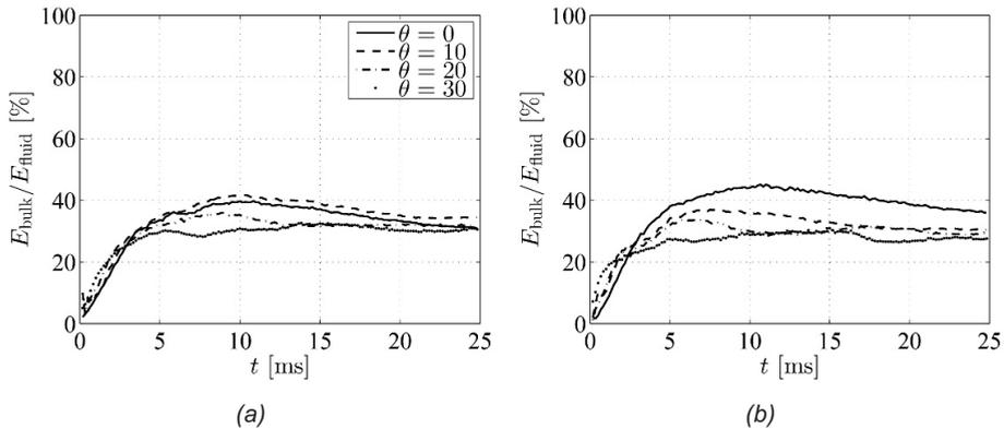
Fig. 5: Average of energy imparted to the fluid bulk  $E_{\text{bulk}}(t)$  calculated as a percentage of the total energy transferred to the fluid  $E_{\text{fluid}}(t)$  for: (a)  $\alpha = 0^\circ$ , (b)  $\alpha = 10^\circ$ . (Figures adapted from [10])
