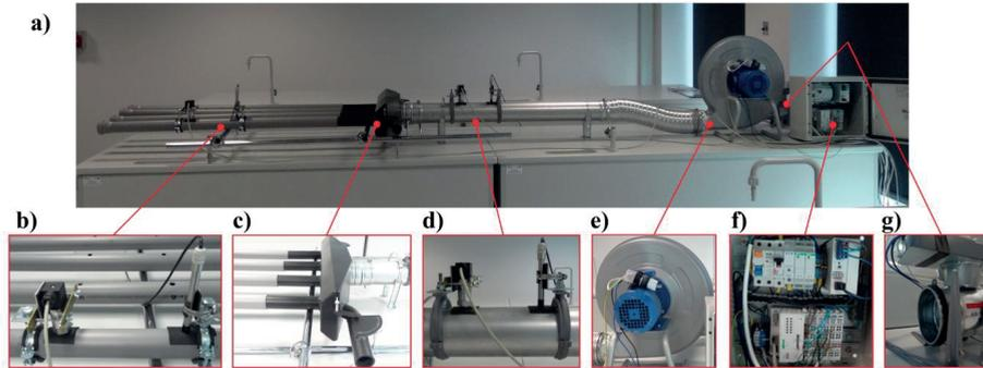
Figure 2. The test stand (a) and selected components: b) the outlet measurement set, c) the examined air manifold, d) the inlet measurement set, e) the centrifugal fan, f) the applied automation, g) the throttle.
