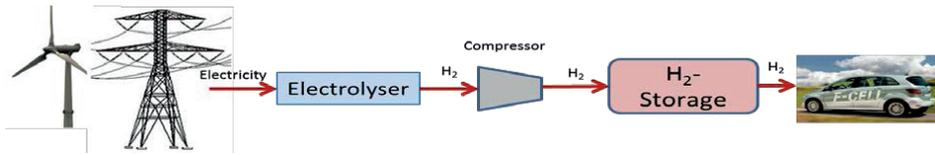
Fig. 6. Energy supply chains: Use of RES in FCVs
