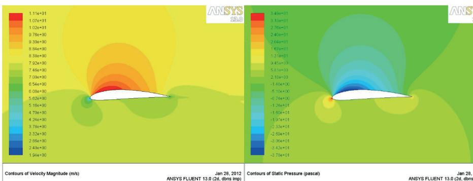
Fig. 4: Contours of velocity (left) and static pressure at designed angles of attack
