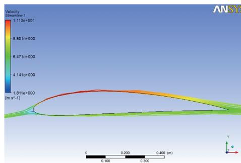
Fig. 5: Velocity streamlines at designed angles of attack
