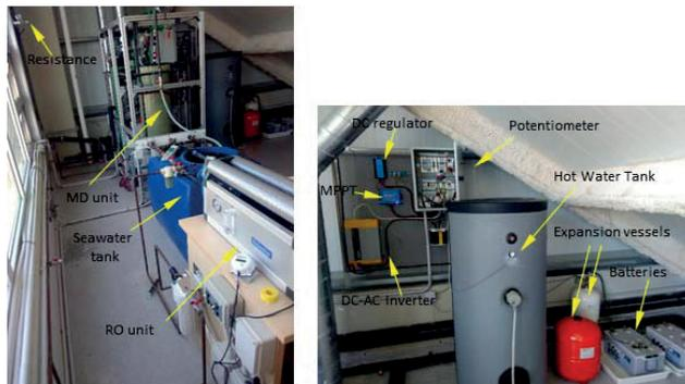
Figure 2.2: Detail of the RO and MD units (left) and electric cabinet, hot water tank and batteries.
