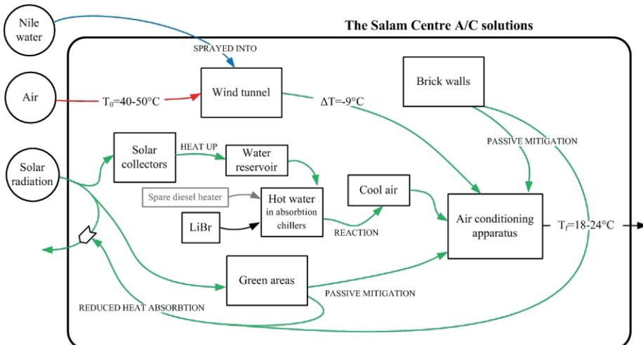
Fig. 4: Scheme describing the Salam Centre solutions for air conditioning through renewables
