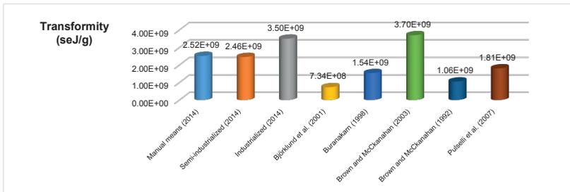
Figure 3.4: Comparison of the transformities of concrete.
