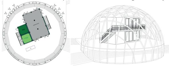
Fig. 2: The Dome has a diameter of 16 metres (200 sqm built area) and in addition to the various open spaces offered inside the greenhouse, a wooden pavilion provides two meeting rooms. The floorplan on the left shows the larger meeting room on the ground floor ("Dome #3), above which the smaller room is located (Dome #2), seen on the perspective. The pavilion in the Dome was designed by the KTH architecture student Stefania Dinea, following a student competition in 2014.<sup>5</sup>
