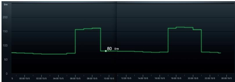
Figure 3.2: As visualized on the in-home display; electricity price forecast (öre/kWh) of the next 24 hours, showing the morning peak period (6-9 a.m.) and afternoon peak period (5-9 p.m.)
