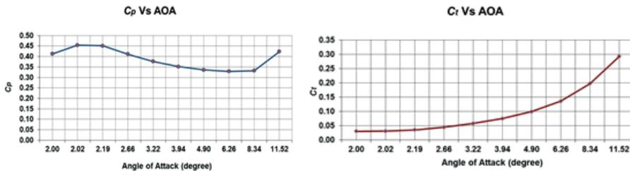
Fig. 3: Power coefficient ( $C_p$ ) (left) and Thrust coefficient ( $C_i$ ) versus angle of attack (AOA)
