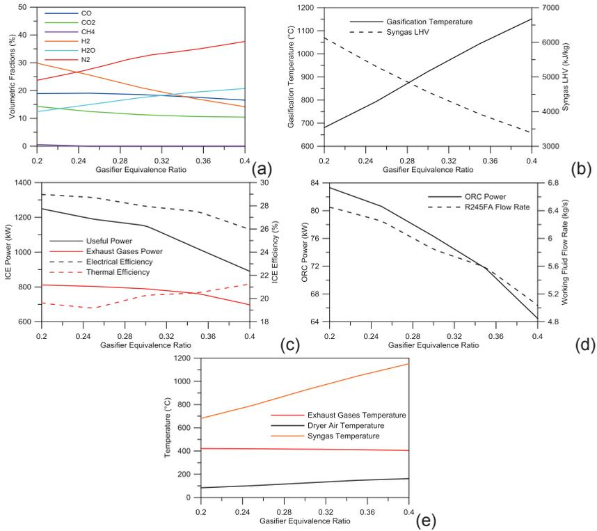
Figure 3.1: Trends as a function of the gasifier equivalence ratio of a) syngas species composition, b) gasification temperature and syngas LHV, c) ICE useful and thermal power, and ICE electrical and thermal efficiency, d) ORC power output and working fluid flow rate, e) exhaust gases, syngas and air dryer temperatures.
