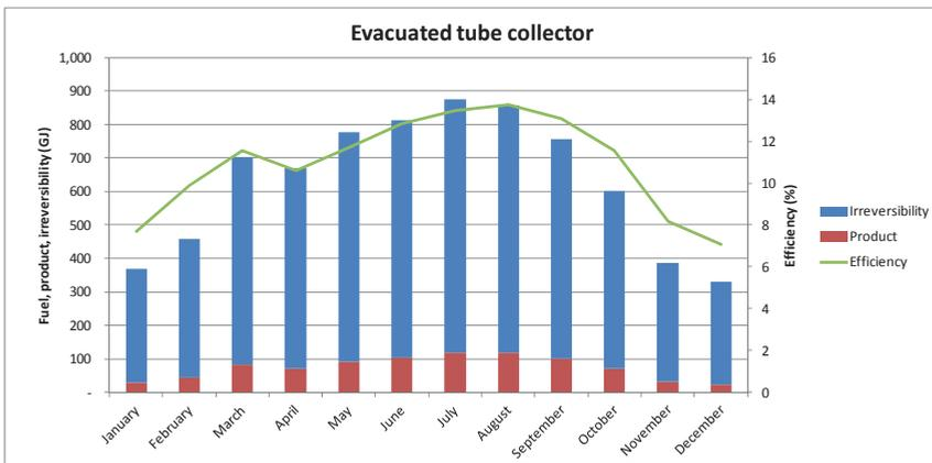
Figure 3.4: Aggregated monthly fuel, product, irreversibility and efficiency of evacuated tube collector.
