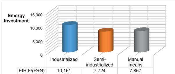
Figure 3.2: Energy Investment Ratio of concrete mixing.
