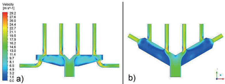
Figure 6. Comparison of the velocity in case of the standard air manifold (a) and the prototype (b): 3D analysis, symmetry plane, inlet velocity of 12.5 m/s.
