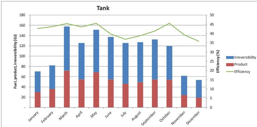
Figure 3.5: Aggregated monthly fuel, product, irreversibility and efficiency of hot water tank.
