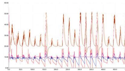
Figure 4. Temperature profile of the collectors, cold medium and hot medium of the installation between hours 0 and 500 of the year (winter period).
