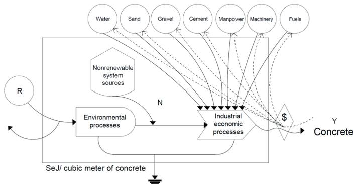
Figure 3.1: Simplified diagram of energy flows in the production of concrete.
