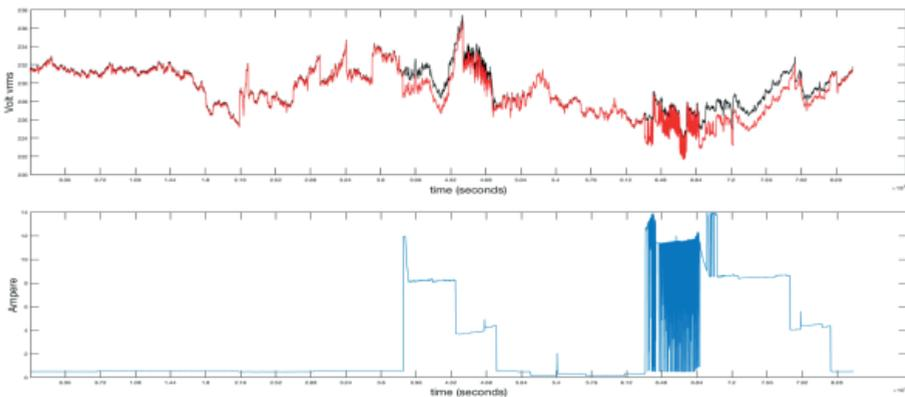
Figure 1: 2016/04/19 00:00-23:28, x-axis in sec: Empirically measured vrms (red), theoretical voltage (black) when calculating the effect of the irms (blue) electric current values due to the EV charging 'away'.
