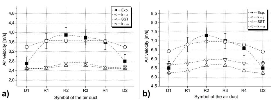
Figure 3. The comparison of results of the experiment and the CFD modelling for selected degrees of the throttle closing with different approaches to the simulation of the turbulence. R1 – R4 – primary air ducts, D1, D2 – secondary air ducts (see Fig. 8). Throttle closing in the given examples: a) 70%, b) 65%, c) 60%, d) 55%.
