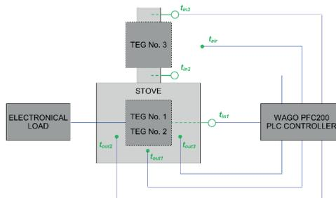
Fig. 1: The general scheme of experimental rig.
