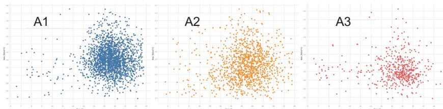
Fig. 2. Distribution of the balance point temperature  $\theta$  (horizontal) and the energy performance coefficient  $\beta$  (vertical) for the constructed archetypes A1 (residential buildings 1946-1975), A2 (office buildings) and A3 (residential buildings 2006-...).
