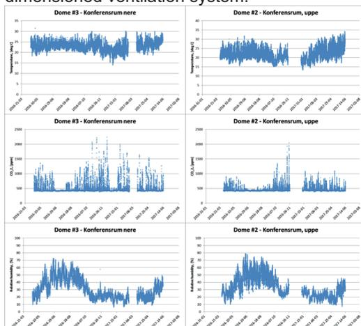
Fig. 4: Long term plot of indoor dry air temperature, relative humidity and CO<sub>2</sub> concentration for the room located in the ground floor of the Dome of Visions (left), and on the first floor (right).
