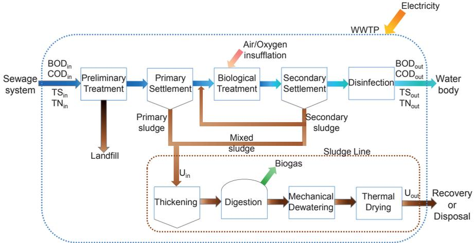
Figure 1.1: Stages of treatment of a conventional WWTP.
