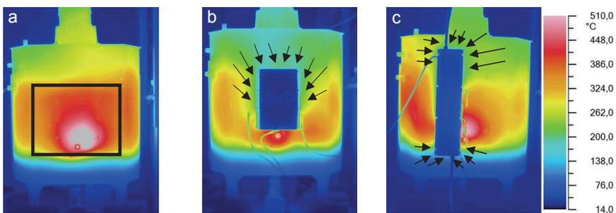
Figure 2: Thermographic analysis of the temperature distribution of the stove's rear surface: (a) without generators, (b) with TEG No. 1 mounted, (c) with TEG No. 2 mounted
