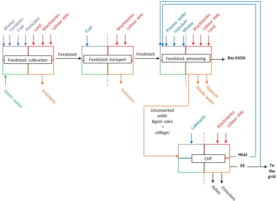
Fig. 2: Processor scheme representation of the studied production system.
