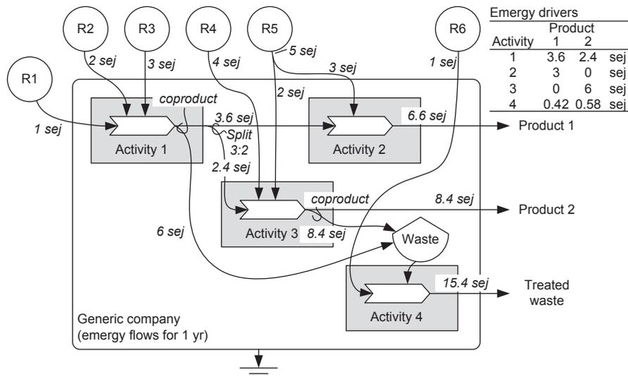
Figure 2. Emergy flows for a generic company to exemplify emergy-based drivers used within ABC-emergy approach. Legend: R = resources.
