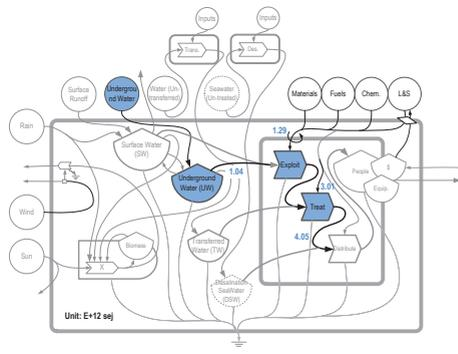
Fig. 3 Emery diagram of ground water treatment (per  $m^3$ )
