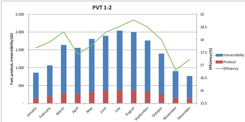
Figure 3.3: Aggregated monthly fuel, product, irreversibility and efficiency of PVT collector 1-2.
