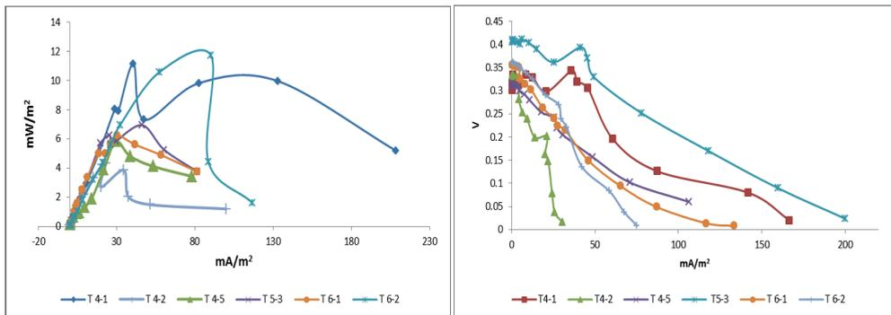
Fig. 5: Polarization and power curves after six weeks of operation at maximum power.
