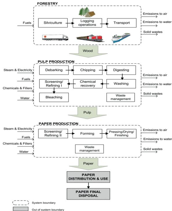
Figure 2.1: System boundaries and process chain under study.
