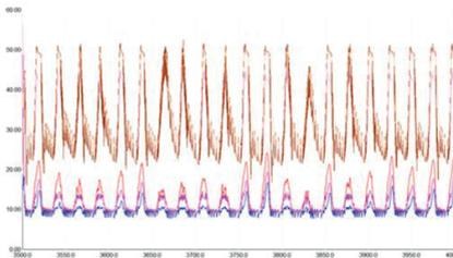
Figure 3. Temperature profile of the collectors, cold medium and hot medium of the installation between hours 3500 and 4000 of the year (summer period).
