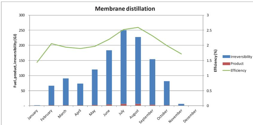
Figure 3.6: Aggregated monthly fuel, product, irreversibility and efficiency of membrane distillation unit.
