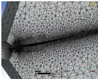
Fig. 2: Concentrated mesh generated around blade and hub surfaces
