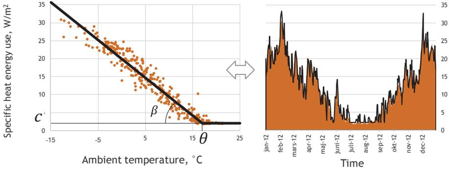
Fig. 1. Example of (left) the energy signature of a building and (right) specific heat energy use by time. Measured and modelled values are coloured orange and black, respectively.
