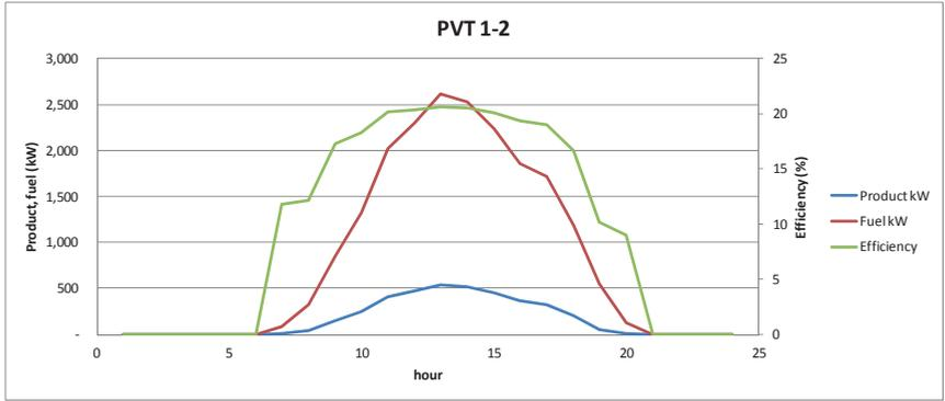
Figure 3.1: Time evolution of fuel, product and efficiency of PVT collector in an example summer day.
