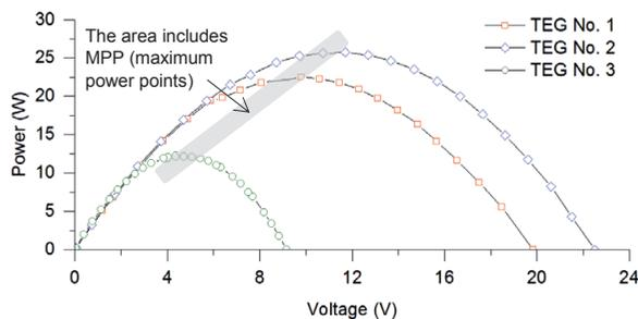
Figure 4: P-V characteristic of the considered thermoelectric generators
