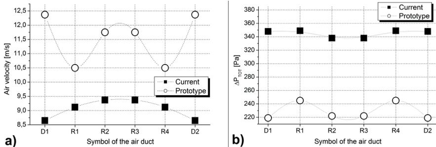
Figure 5. Distribution of selected outlet parameters in case of the basic air manifold and the prototype, inlet air velocity of 12.5 m/s
