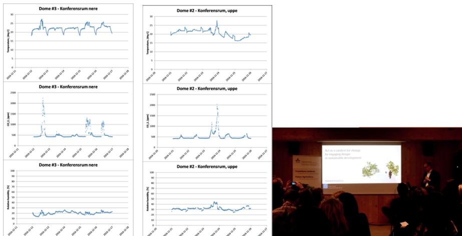
Fig. 5: Plots of indoor dry air temperature, CO<sub>2</sub> concentration and relative humidity for the week 12-17/12/2016, to the left the room on the ground floor Dome #3. Centre, the room on the first floor, Dome #2. To the right we see how, on 12/12/2016 the larger meeting room was filled with 56 seated guests and 14 standing guests between 2-6PM<sup>6</sup>. This even was preceded by a lunch talk by the “Centre for Land Use” with 20 participants 12-13PM.<sup>7</sup>
