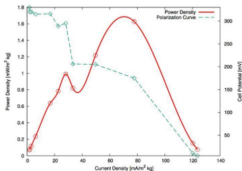
Fig.2: Power and polarization curves after 3 weeks of operation.
