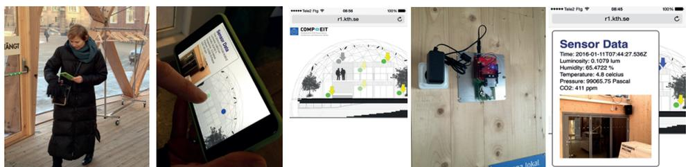
Fig. 3: A basic web interface gives visitors easy access to real-time sensor data. Experimental weather stations have been placed in different locations inside the Dome of Visions.
