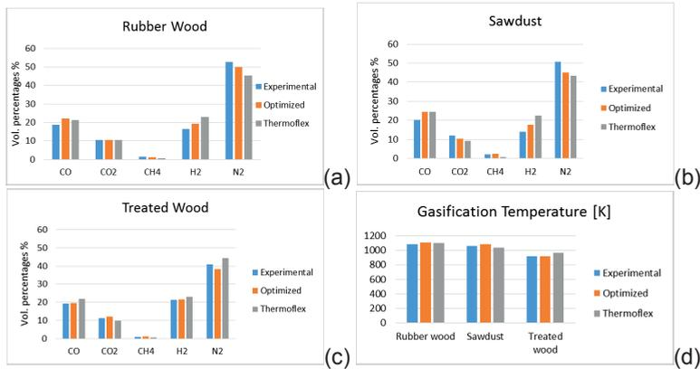
Figure 2.2: Comparison between experimental measurements, numerical results of both the optimized equilibrium model and the Thermoflex™ model in terms of volumetric syngas compositions for a) rubber wood, b) sawdust, c) treated wood and d) gasification temperature.
