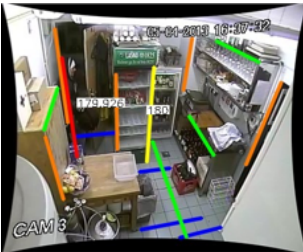
Figure 2. Calibration of a room should be performed after image distortions are corrected. The figure of the person in the corresponding video is never seen in its entirety. To be able to establish the height of the person, comparison to other calibrated lengths in the image is used.
