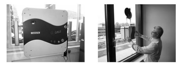
Figure 2: First prototype of the  $U_g$ -value sensor (left) and field test with anti-fall guard (right).
