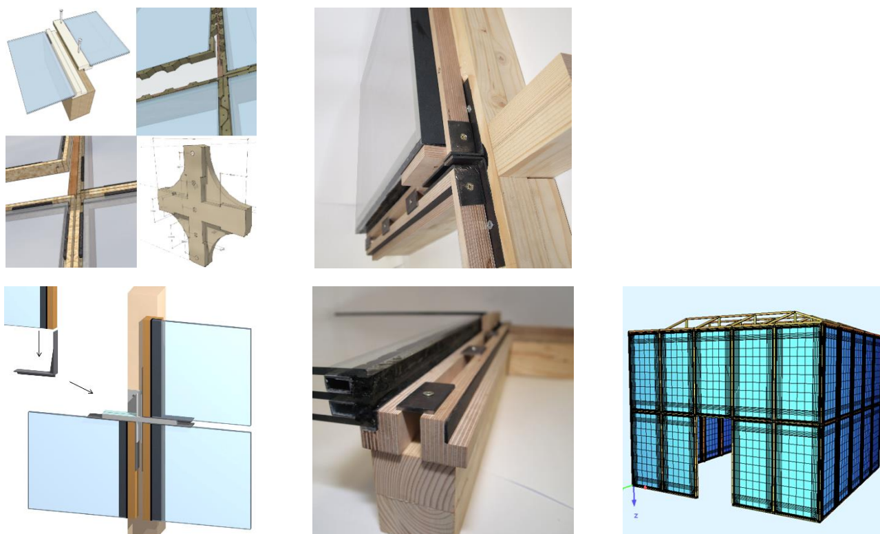
Figure 6: Details of various developed adapter frames and FEM model (ITI [10] and [11])
