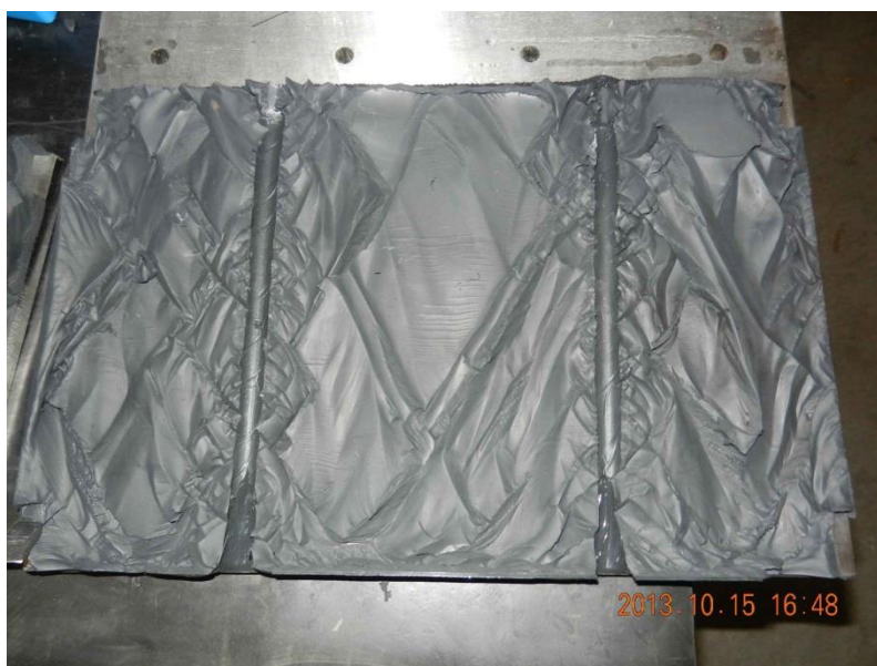
Figure 6: Test sample after the approved test: the failure mode is cohesive.
