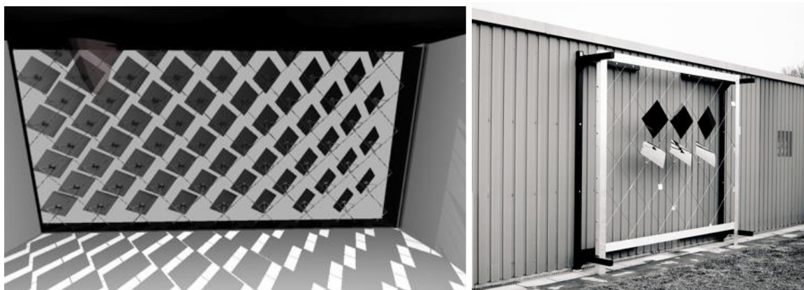
Figure 8: (left) Indoor rendering of the ASF, (right) Prototype with six panels and an aluminium frame. A photovoltaic panel will be mounted at each cable intersection.
