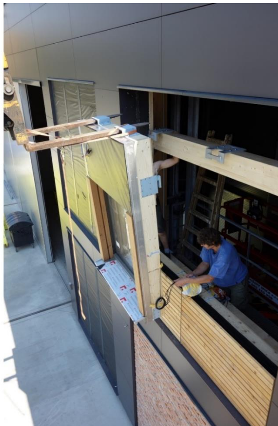
Figure 4: Panels equipped with sensors placed in one of 6 openings in climatic room for long-time observation under conditions close to reality
