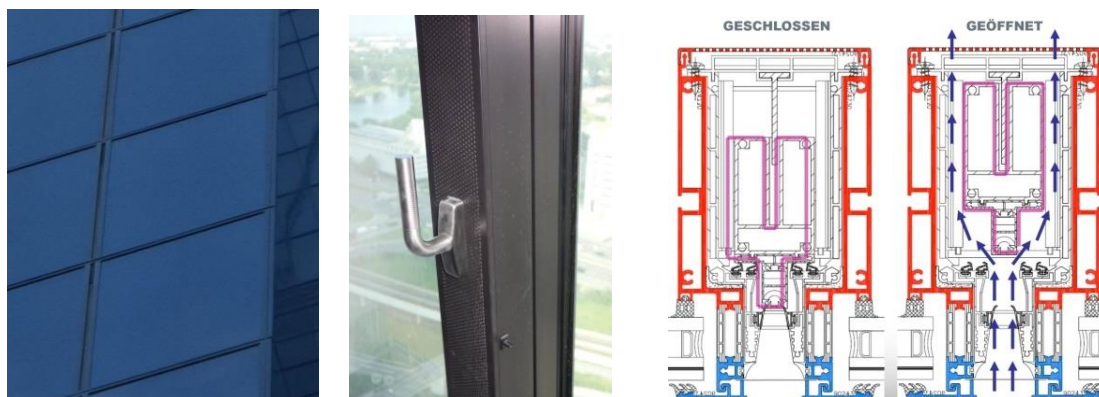
Figure 3: Frame integrated ventilation, DC Tower, Vienna. Source: K. Kizilaslan, L.B. Toprak [7]
