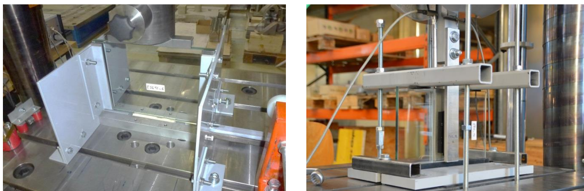
Figure 7: Compressive test performed on contact connections between glass and steel with a resin-based grout and with a thermoplastic (left); shear test on adhesive connections between glass and stainless steel (right).
