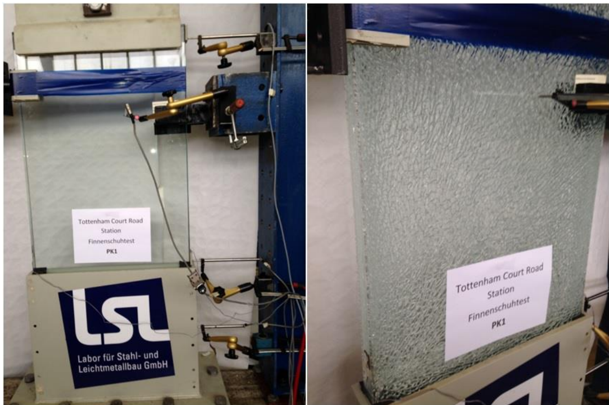
Figure 6b: Testing connection points in the glass fin
