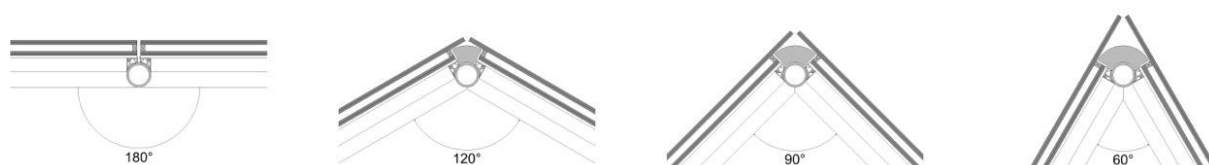
Figure 4: The length of the stepped glazing is dependent on the angles of the design geometry
