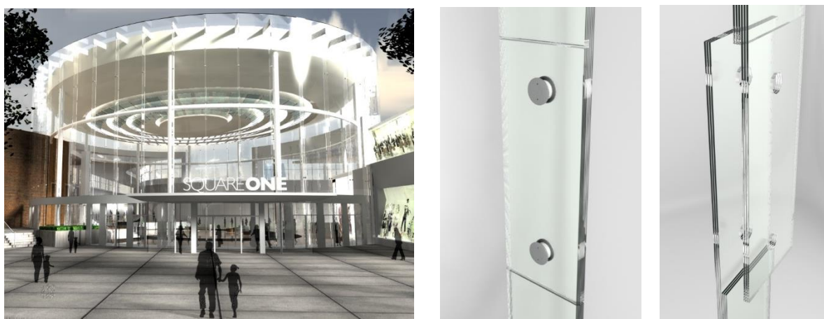
Figure 8: Rendering Rotunda glass fin façade , Square One Shopping Center © Read Jones Christofferson (left); Rendering half lap splice joints glass fin © Read Jones Christofferson (right)
