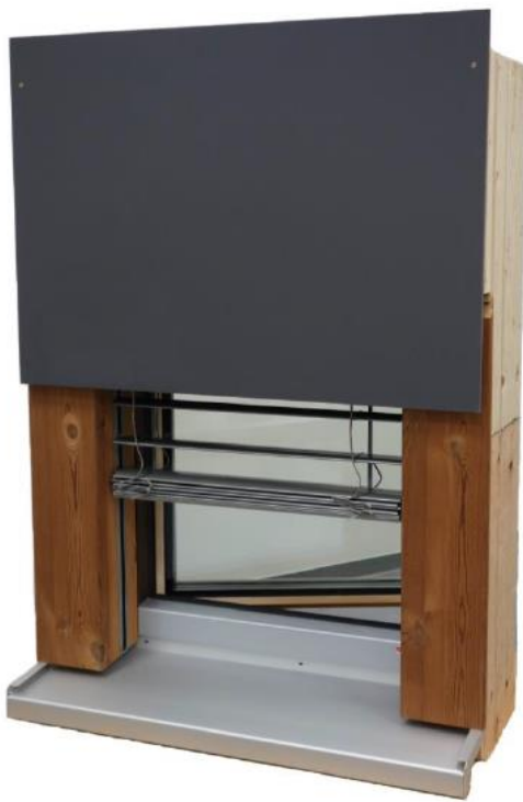
Figure 3: Prototyping - Left: Model for development studies (Thermowood, cement based boards, venetian blinds integrated). Right: Placing of vacuum insulation boards into full scale prototype
