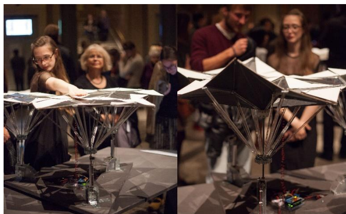
Figure 6: Floral Skin in winter mode (left) and summer mode (right). (picture courtesy MAK/K.Wißkirchen)
