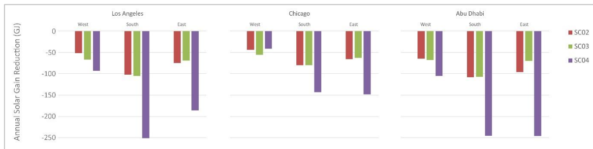
Figure 27: Different shading strategies' annual solar gain reduction compared to the benchmark scenario.
