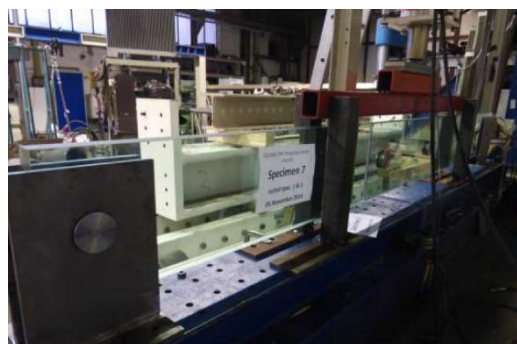
Figure 10: Test Set-up half lap splice joints (left) and test assembly overview (right)
