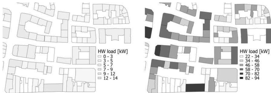
Fig. 3.1: Hot water loads with simplified (left) and detailed (right) model
