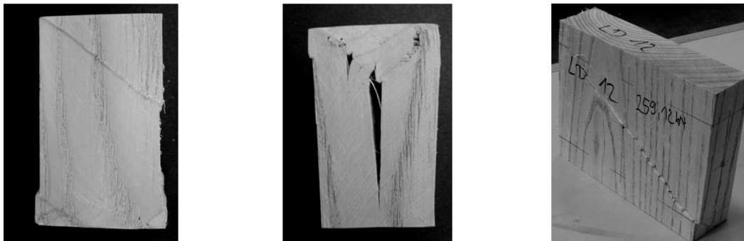
Fig. 4.14: Specimens of Tree-of-Heaven ( Ailanthus altissima (Mill.) Swingle) which failed in compression parallel to grain: clear wood with 45° inclined shear band in tangential direction (left) and with formation of a shear wedge followed by tension failure perpendicular to grain (middle); structural timber specimen with shear band in roughly 45° in tangential direction (right)
