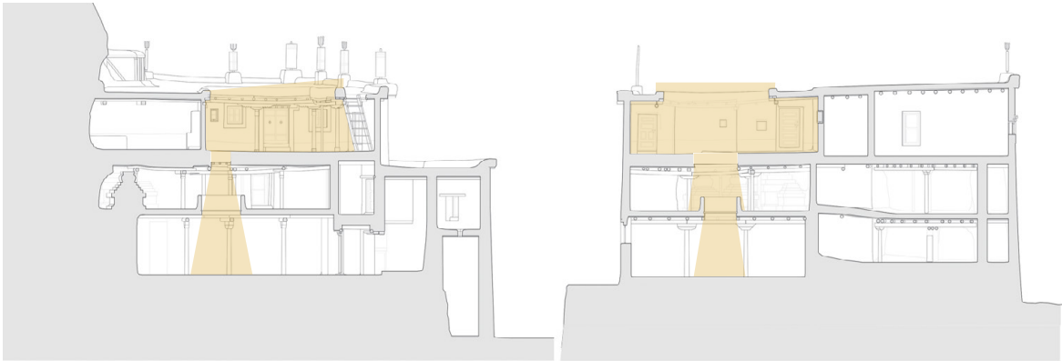
283 Conception of a glass roof above the inner courtyard and the reopening of the skylights on the second and third floor. TU Graz 2013.
