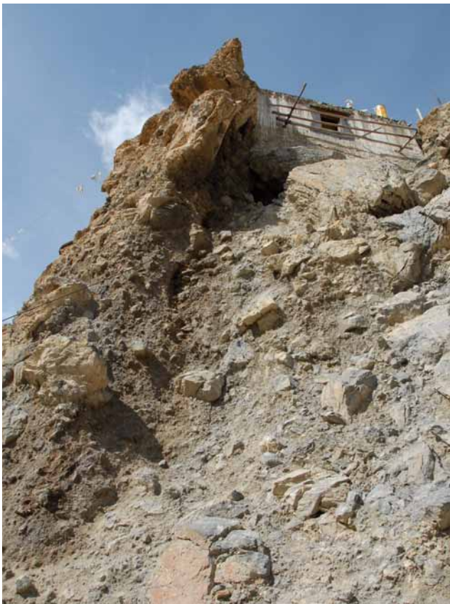
215 Typical characteristics of the bimrock materials forming the cliffs of Dangkhar. K&S 2011.
