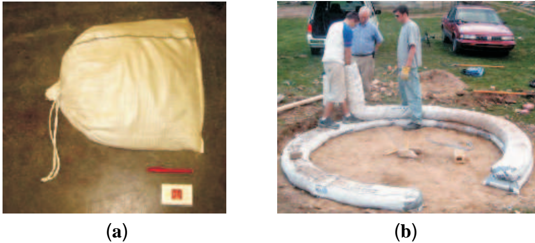
Figure 1.4: Typical shapes of soilbags for instance for: (a) foundation of buildings and roads, (b) for dome.
