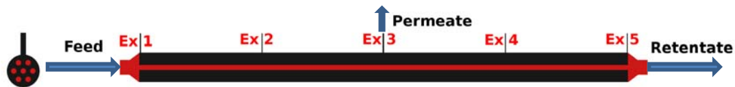
Figure 1: Seven fiber module geometry and exit positioning at permeate side (scaled 1:10 in length)
