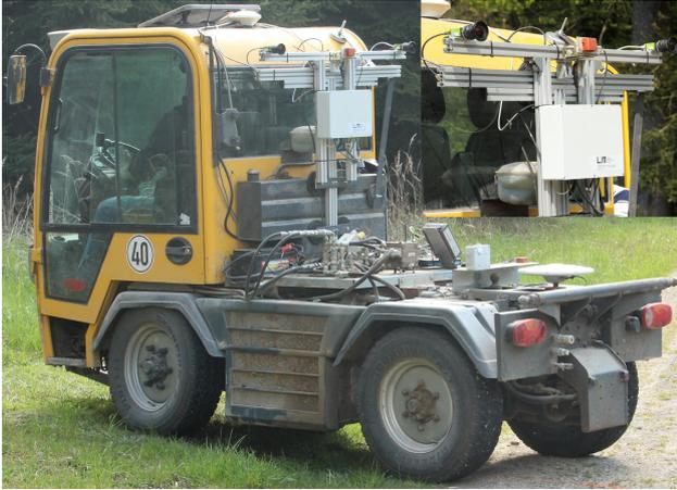
Fig. 2: Vehicle with measurement setup and DGPS-receiver
