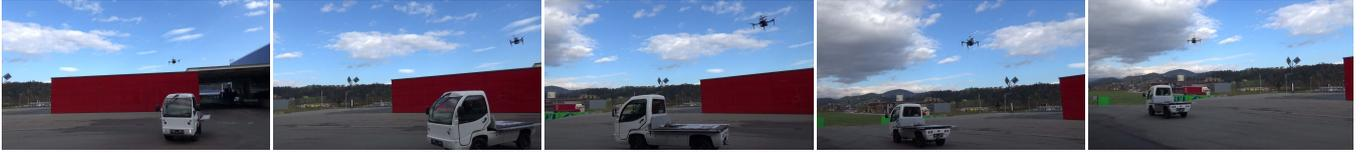
Fig. 3. Drone vision-based vehicle following, marked with a  $39 \times 39$  cm Apriltag. Experiment: 3 min, mean speed 7.91 km/h and top speed 13.35 km/h.
