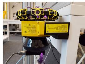
Fig. 3. Example of a problematic setup where 3 different types of sensors are mounted just next to each other. This setup increases the chance of perception failure due shadowing effects and local hazards such as physical damages.
