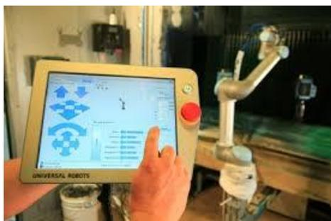
Fig. 2 - www.zacobria.com - UR10 programming
