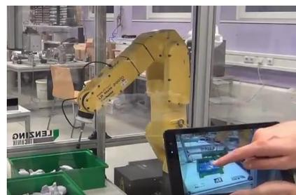
Fig. 14 - 2D tap based process point selection (<https://www.youtube.com/watch?v=nrhXEqG014o>)
