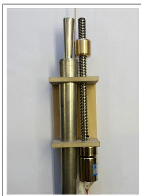
Fig. 6. First prototype with gearbox motor
