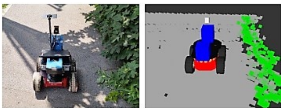
Fig. 7. Detection of the grass through the laser scanner [5].
