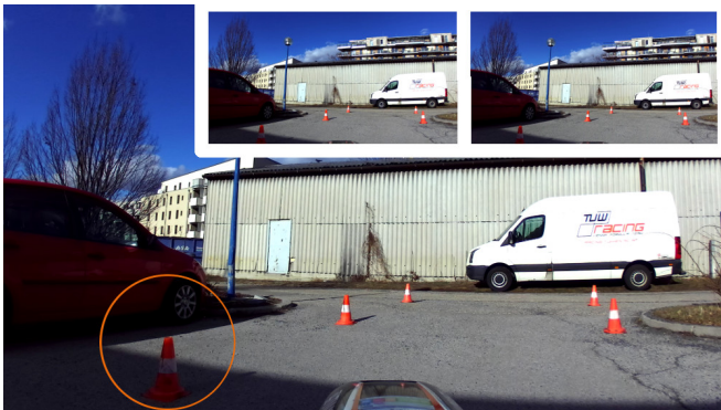
Fig. 7. Images of the ZED stereo camera showing how light conditions affect the visual cone appearance.
