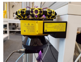
Fig. 3. Example of a problematic setup where 3 different types of sensors are mounted just next to each other. This setup increases the chance of perception failure due shadowing effects and local hazards such as physical damages.
