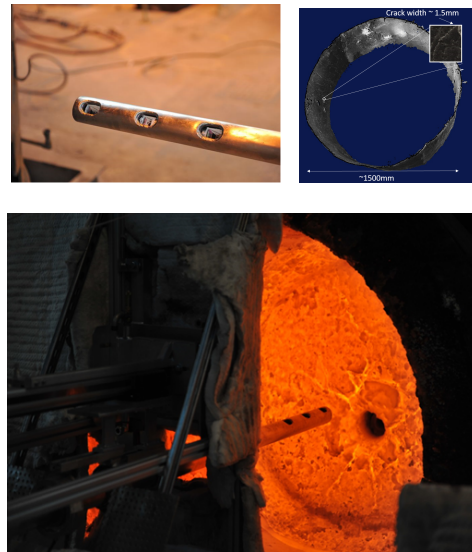
Fig. 3: Stereo system with active speckle projection for the inspection of red hot steel components, ladles and chambers with up to 1.600°C. ©Materials Processing Institute supported by Dr BG Crutchley of i3D robotics Ltd.
