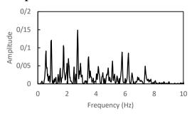
Figure 7-PSD spectrum of horizontal component of Kobe far field motion
