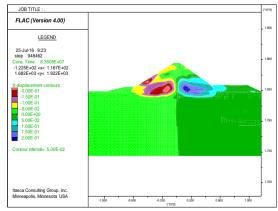
Fig 7. Vertical displacement contours (m)
