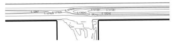
Figure 6. The contours of free surfaces for p = 0.1 m, L = 0.5 m, Fr = 0.42
