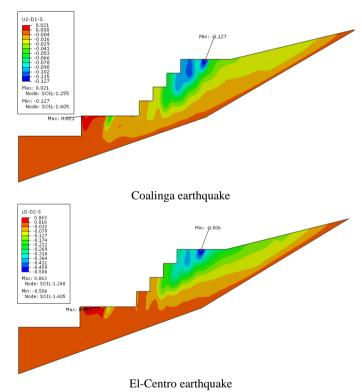
Figure 7. Contour of horizontal settlement of walls
