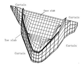
Figure 3. Finite element mesh of the anti-seepage system.
