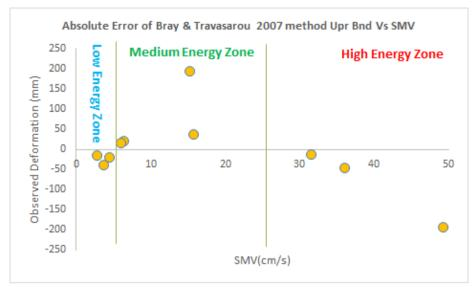
Figure 4. The absoluteerrors of the upper bound values of Bray and Travasarou 2007 coupled-based method (the designee method), for estimating max deviatoric deformations versus SMV of the Group 1 case studies
