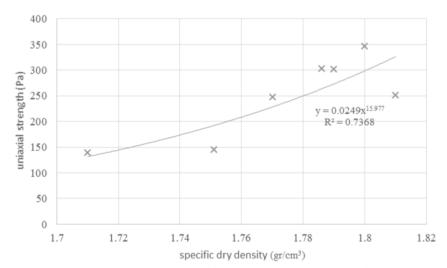
Fig 1: Uniaxial strength versus specific dry density in unreformed specimens
