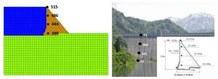
Figure 2 Geometry of the 2D model compare to the gravity dam
