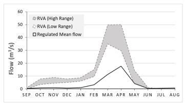
Figure 2. Comparison of the mean flow of Gadar River after operation of the Hasanlu Dam to the flow range proposed by the RVA method as environmental flows of the river.
