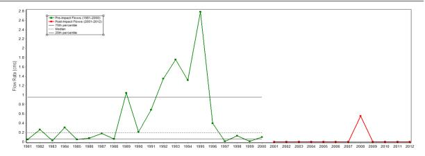
Figure 7. Comparison of the 7-days Minimum flows before (green line) and after (red line) the dam operation.
