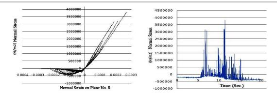
Figure 7 a) normal stress vs. strain, b) time history of Normal stress on plane no. 8 of Node 85
