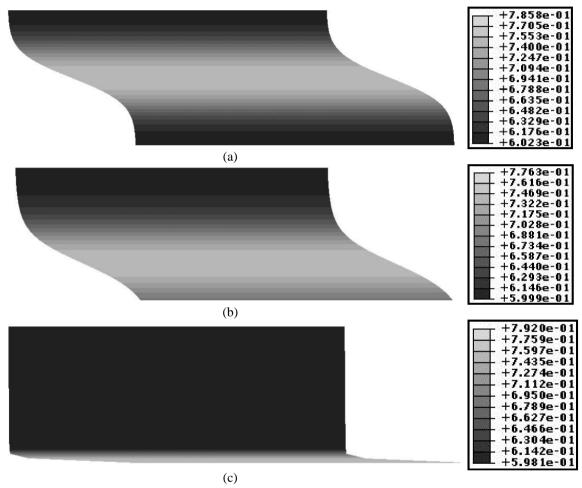
Figure 5. Deformed shape of granular soil layer along with contour plot of void ratio after  $U_{IB}/h_0 = 1.00$  for: (a) Case (1):  $f_T = 0$  and  $f_B = 0.0001$ , (b) Case (2):  $f_T = 0$  and  $f_B = 0.01$  and (c) Case (3):  $f_T = 0$  and  $f_B = 0.5$
