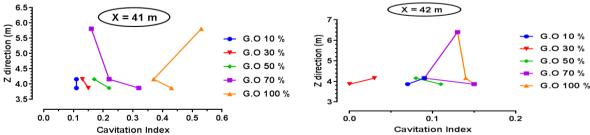
Figure 17. Cavitation index variation on the conduit wall for the different service gate opening at section of 41m from the conduit entrance
