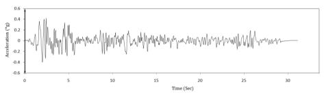
Figure 2. Time history of base reference input acceleration, (El-Centro earthquake, 1940)
