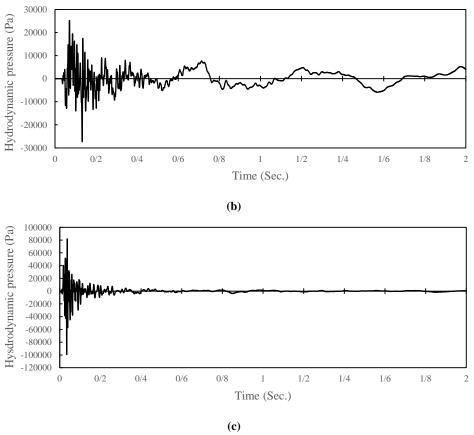
Figure 10-time histories of hydrodynamic pressure in dam heel. A) Explosion near to dam crest. B) Explosion at the
