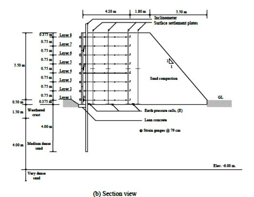
Figure 2. Schematic diagram of the test wall instrumentation
