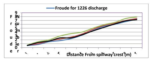
Figure 3- The comparison of Froude number changes over the spillway of Azad dam for critical discharges
