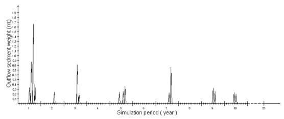
Figure 3.5. Density-current outflow sediment at SAMP Reservoir
