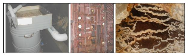
Figure 14: Device for collecting sediments from drainage water (design A. Pujol), severe corrosion of piezometer panel by aggressive water, incrustation with carbonate and manganese precipitate.
