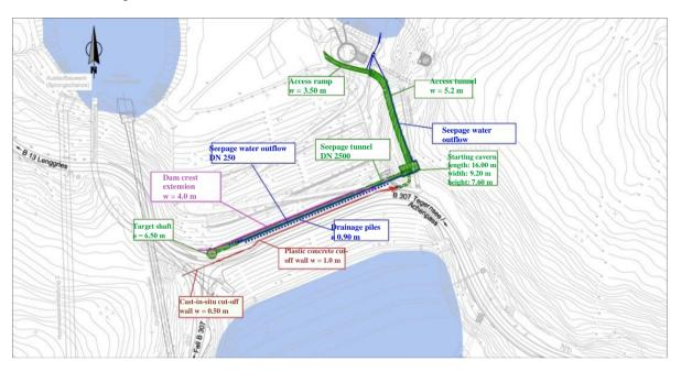
Figure 1. Layout of the rehabilitation concept (Source: WWA-WM)
