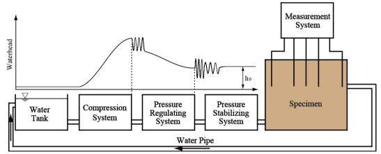
Fig.2 Principle of the in-situ seepage test
