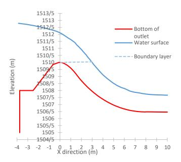
Figure 7:Flow pattern for Q=501.5 m3/s
