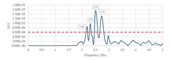
Figure 7- first singular value of recorded motion
