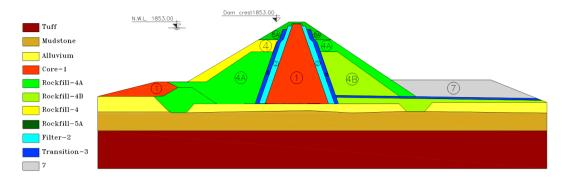
Fig 1. Typical cross section of Ghoocham dam
