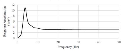
Figure 3- Spectral Acceleration of Type 1 Earthquake (Peak Acc. Equal to 0.3g)
