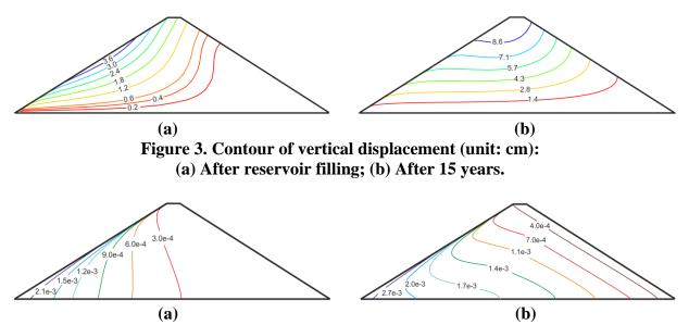
Figure 4. Contour of reduction of the void ratio: (a) After reservoir filling; (b) After 15 years.
