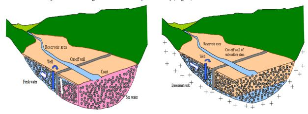
Figure 6. Dam up type (storage type), Saltwater intrusion prevention type [14].
