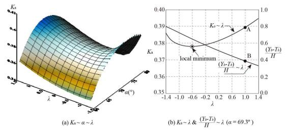
Fig. 6. The variation of the active earth pressure and its application point with  $\alpha$  and  $\lambda$  (based on nonlinear strength parameters:  $\varphi_0 = 45^\circ$  and  $\Delta \varphi = 8^\circ$ )
