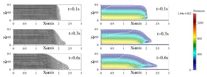
Figure 1. Mudflow profile in dam-break problem; left column is studied by [5]; right column is the present study
