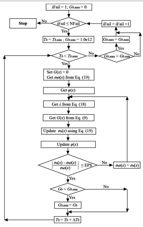
NFail: number of failure surfaces considered;  $T_{b,min} & T_{b,max}$ : lower and upper bounds of  $T_{b}$ ;
