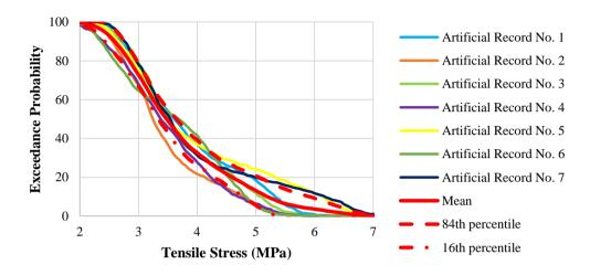
Figure 3. Exceedance probability curves for artificial records applied to the finite element model
