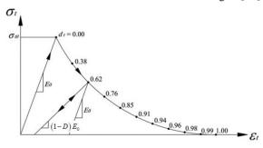
Figure 3. stress-strain relation for the nonlinear concrete
