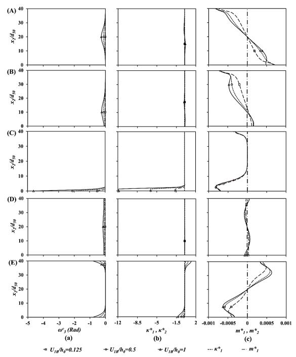
Figure 3. Distribution of (a)  $\omega_3^c$ , (b)  $\kappa_{1,2}^*$  and (c)  $m_{1,2}^*$  across  $x_2/d_{5\theta}$  at different  $U_{1B}/h_{\theta}$  for: (A) Case (1):  $f_T = 0$  and  $f_B = 0.0001$ , (B) Case (2):  $f_T = 0$  and  $f_B = 0.01$  and (C) Case (3):  $f_T = 0$  and  $f_B = 0.5$
