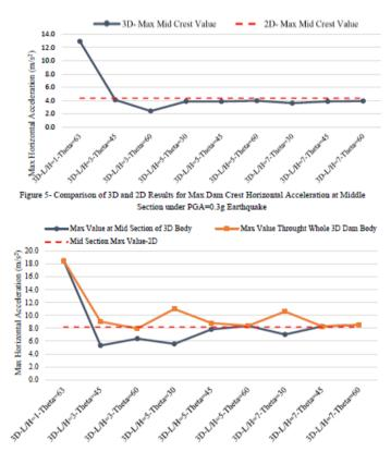
Figure 6- Comparison of Max Horizontal Acceleration Value at Different Locations of Dam Body for 3D and 2D Analysis under PGA=0.3g Earthquake
