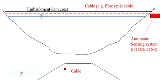
Figure 4: Cable based warning system [4]
