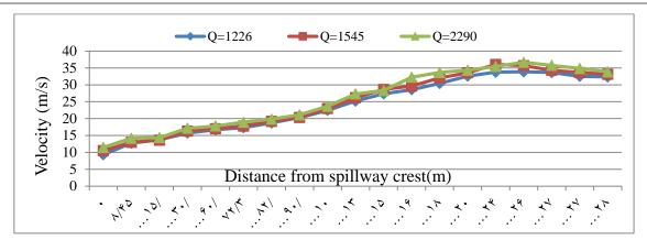
Figure 6- The comparison between numerical velocity for three discharges (1226, 1545, 2290 m<sup>3</sup>/s)
