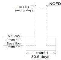
Converting monthly av. flow (mcm/m) to instantaneous flood discharge (cms)
