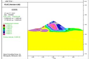
Fig 15. Vertical displacement contours (m)
