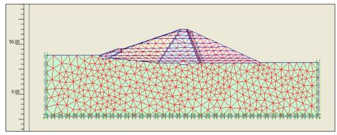
Figure 4. The finite element model of the embankment
