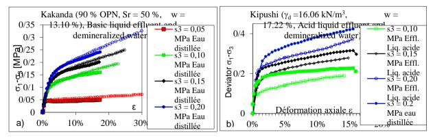
Figure 5. Diagram deviator - axial deformation in CU
