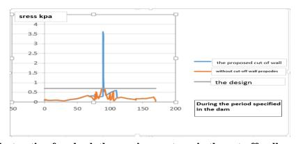
Figure 7. selectsection for check the maximum stress in the cut-offwall proposed 100 cm
