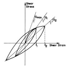
Fig 2. Nonlinear cyclic stress-strain relationship of soils [1]
