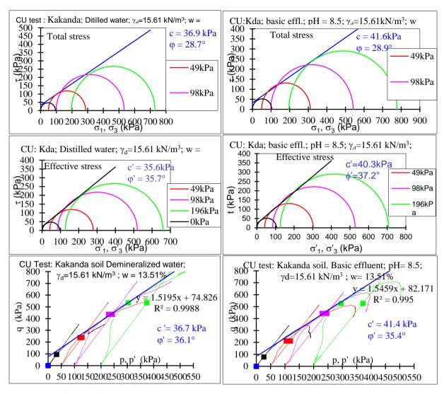
Figure 4. Circle of Mohr, intrinsic right, and critical state line for the soil of Kakanda.
