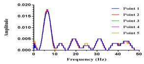
Figure 19. hydrodynamic pressure power spectrum for 20% gate opening
