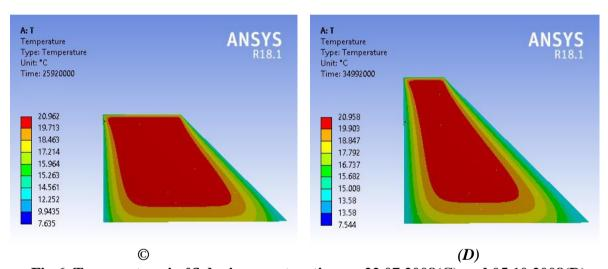
Fig.6. Temperature in °C during construction on 22.07.2008(C) and 05.10.2008(D)
