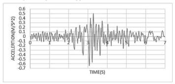
Figure 2. Manjil earthquake scaled horizontal accelerogram (PGA0.5)
