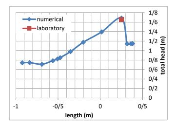
Figure 5. Numerical & Laboratory mound at Q=0.091 cmps
