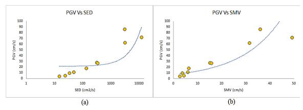
Figure 8. PGV versus energy representative parameters for Group 1 earth dams
