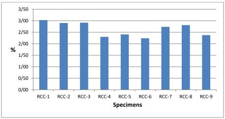
Figure 4. 24-houre water absorption
