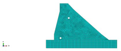
Figure 3. Meshing by finite element analysis of Zavin concrete gravity dam
