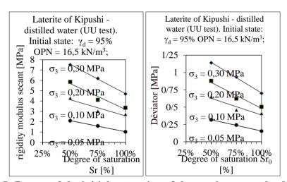
Figure 9. Influence of the initial saturation of the specimens on the deviator and the secant modulus of rigidity
