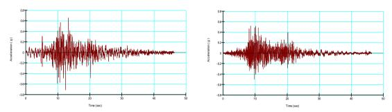
Figure 3. Horizontal (left) and vertical (right) acceleration time history (Tabas) in SEE level
