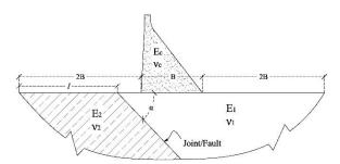
Figure 2. Inhomogeneity of the foundation
