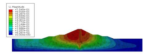
Figure 8. Total Vertical Displacements at the End of Construction Stage Considering the Sealing Wall Implementation up to the Crest Level
