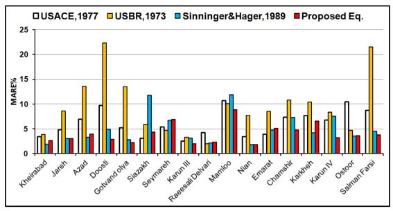
Figure (5)- Evaluation of different methods for the discharge estimation of spillways with radial gate
