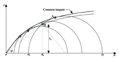
Fig. 12. The strength envelope based on triaxial experiments
