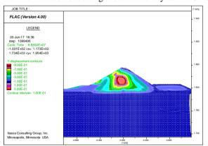
Fig 11. Vertical displacement contours (m)
