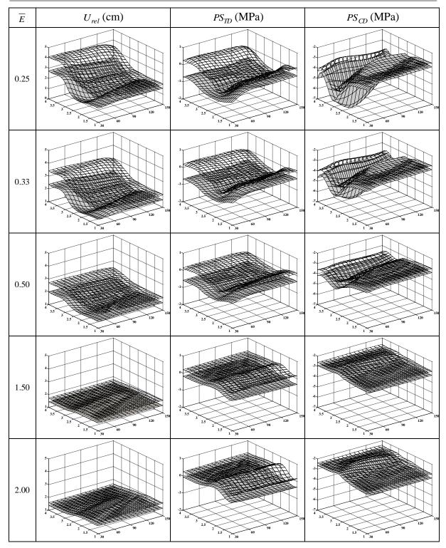
Figure 3. The results of the one-fault models. The second, third and fourth column respectively show the  $U_{rel}$ ,  $PS_{TD}$  and  $PS_{CD}$  for the dam body in terms of I/B (left horizontal axis),  $\alpha$  (right horizontal axis) and  $\overline{E}$ . The filled and un-filled curves are representing the models under the loading combination LC1 and the LC2, respectively.
