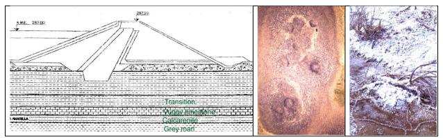
Figure 9: Casa de Piedra Dam, geological section of foundation, boils, efflorescence
