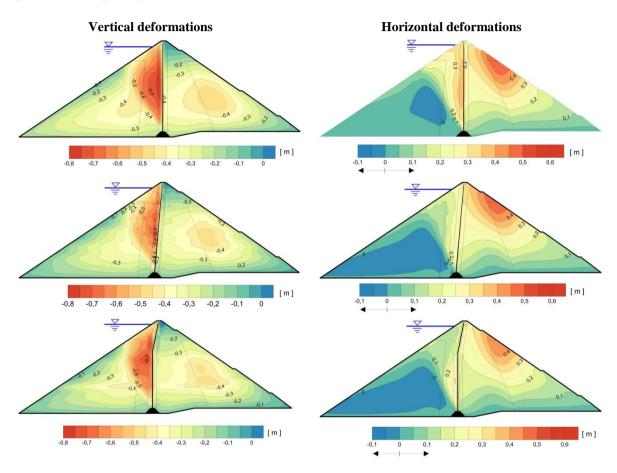
Figure 8. Vertical and horizontal deformation
