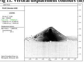
Fig 13. Displacements vectors (m)
