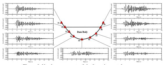
Figure 9. North components of the 9 receivers at dam canyon
