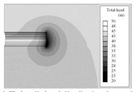
Figure 4. Hydraulic head distribution thorough model
