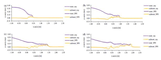
Figure 5. Free surface and bed surface changes on PVC bed study at t=0.25, 0.50, 0.75, 1.0s (compared with [2])
