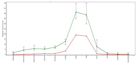
Figure 6. Mean Monthly Flow of the Gadar River during pre (green) and post-dam period (red line).
