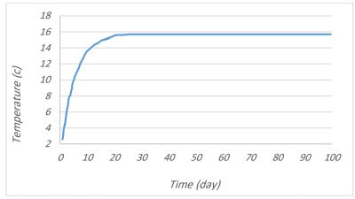
Fig.1.Adiabatic temperature rise due to hydration heat.
