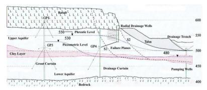
Figure 13: Drainage system in buried valley under left abutment of Piedra del Águila
