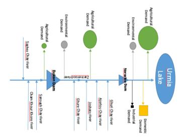
Figure 3. A schematic view of water inflows and withdrawals to the Zarinerood River downstream of Bukan Dam
