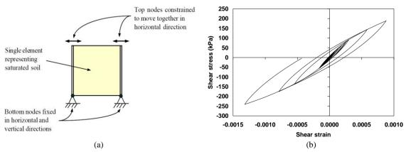
Figure 6. Simulation of cyclic simple shear test of one-zone sample in FLAC: (a) applied boundary conditions, and (b) Hyteresis loops
