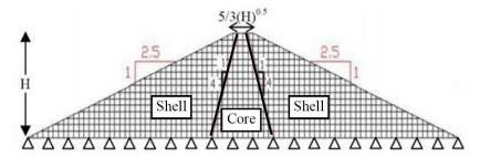
Figure 2. Geometry of dam
