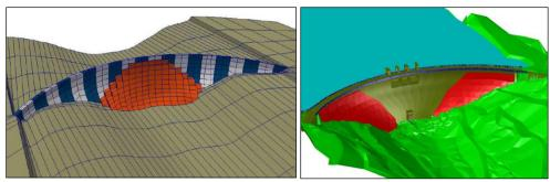
Figure 5 central and lateral downstream reinforcement of the dam.
