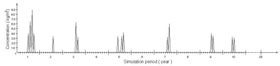
Figure 3.4. Density-current outflow concentration at SAMP Reservoir
