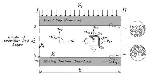
Figure 1. Modeling plane shearing of granular material under constant vertical pressure: section of extended infinite granular soil layer located between two parallel rigid boundaries of varying surface roughness along with kinematics and static quantities of micro-polar material under plane strain condition
