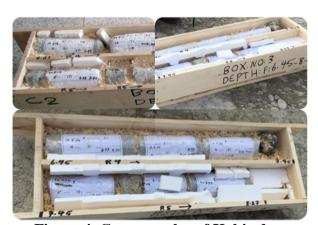
Figure 4. Core samples of Kahir dam
