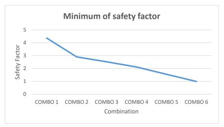
Figure 6. The minimum of safety factor of wedge for different load combination
