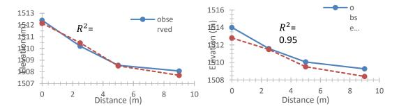
Figure 3: Comparison of observed and simulated surface water elevation for Q=501.5 m3/s
