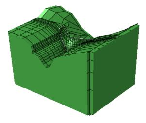
Figure 3. Finite element model of Luzzone dam
