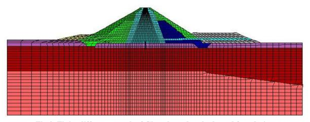
Fig 2. Finite difference mesh of Ghoocham dam body and foundation
