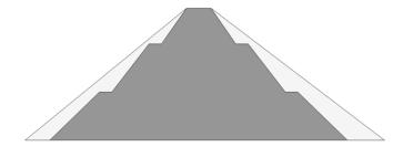
Figure.1. Employing berms in order to reduce fill volume in earth dams
