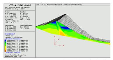
Figure 7. The G/Gmax ratio contours at the end of equivalent linear analysis
