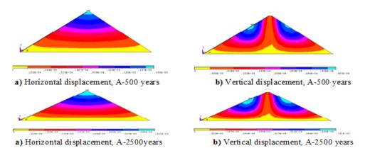
Figure 8. Distribution of displacements in different site class for 500 years returns earthquake period
