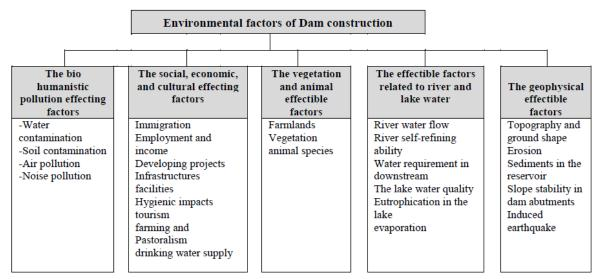
Fig.1- EIA diagram for dams
