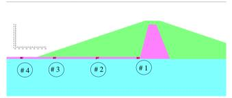
Figure 6. The location of defected zone that hydraulic gradient is measured
