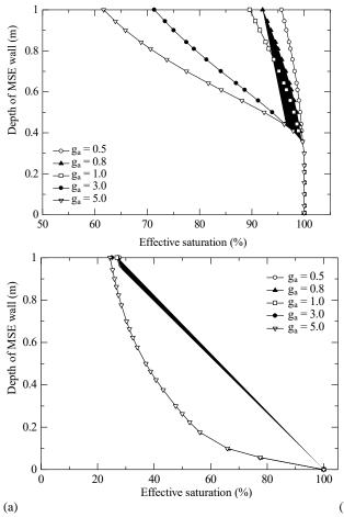
Figure 5: Effective saturation profile along vertical sections located (a) 5 cm left and (b) 5 cm right of the geocomposite for various magnitudes of  $g_a$  of outer soil
