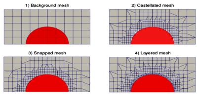
Figure 1. Grid generation steps with the native OpenFOAM meshing tools: a) blockMesh grid, b) snappyHexMesh castellated, c) snappyHexMesh snapped, d) snappyHexMesh addLayers
