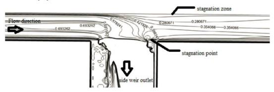
Figure 7. Velocity contours on the free surface for p = 0.1 m, L = 0.5 m, Fr = 0.42
