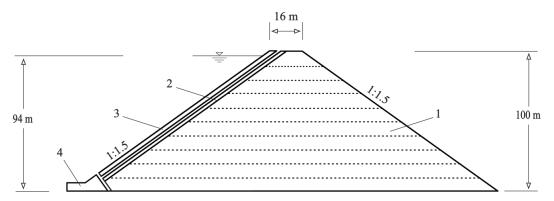
Figure 1. Sketch of the cross section of the CFRD: <1> main rockfill; <2> transition layer <3> concrete slab layer; <4> concrete toe slab.
