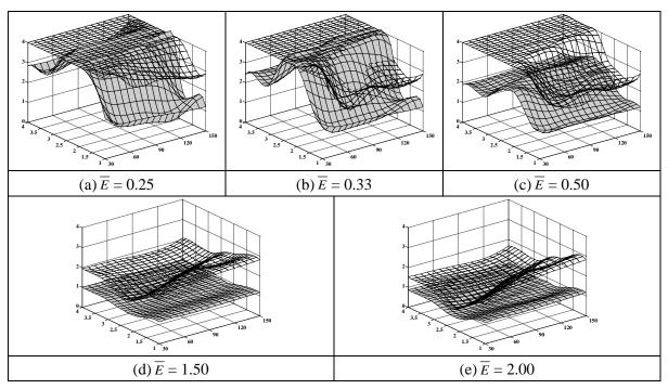
Figure 4. The local sliding safety factor at the dam heel in terms of I/B (left horizontal axis),  $\alpha$  (right horizontal axis) and  $\overline{E}$  ratio. The filled and un-filled curves are representing the models under the loading combination LC2 and the LC1, respectively.
