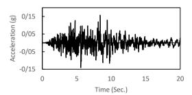
Figure 8-Vertical component of Kobe far field motion
