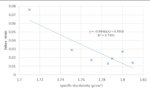
Fig. 2: Failure strain versus specific dry density in unreformed specimens
