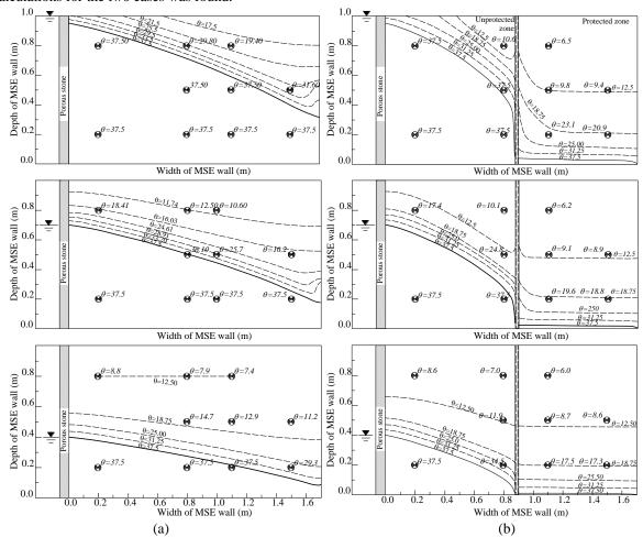
Figure 4 Measured and calculated phreatic surfaces and water contents for MSE wall
