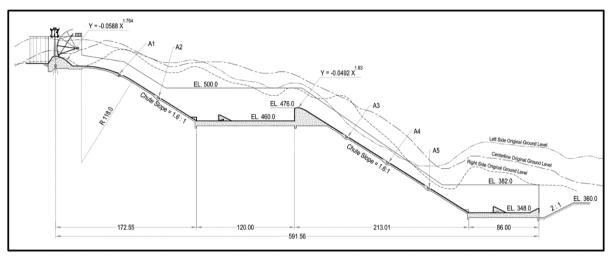
Figure 5. Profile of the spillway
