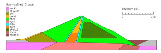
Figure 3. Cross section of the dam in two dimensional analyses
