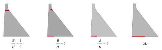
Figure 11. Tensile damage in the highest monolith of 3D and 2D models
