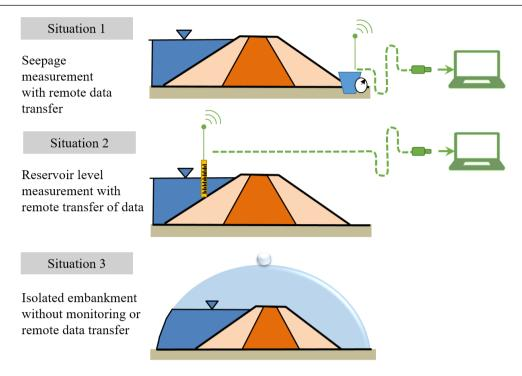
Figure 1: Embankment dam with three different monitoring plans
