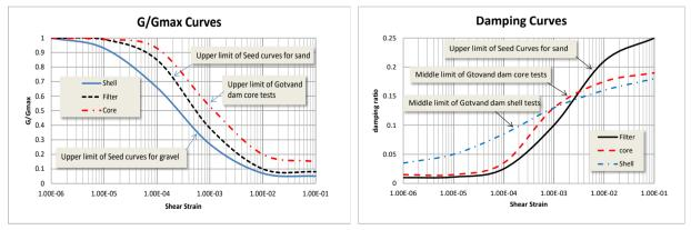
Figure 5. Damping ratio and G/G<sub>max</sub> versus cyclic shear strain
