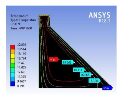
Fig.9. Temperature in °C during construction on 27.01.2009.
