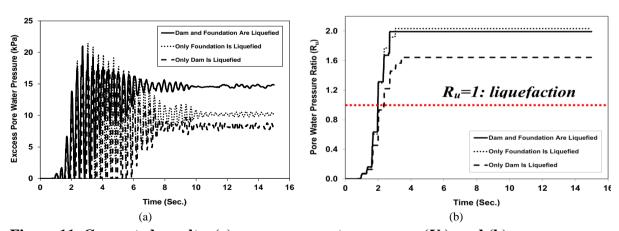
Figure 11. Computed results: (a) excess pore water pressure  $(U_e)$ , and (b) excess pore water pressure ratio  $(R_u)$  time histories at the zone of liquefaction
