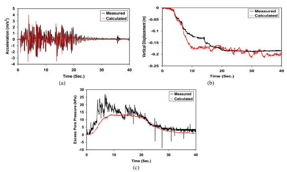
Figure 6. Comparison between obtained numerical results and centrifuge test data: measured versus calculated (a) acceleration time histories, (b) displacement time histories, and (c) excess pore pressure time histories at the middle of dam height
