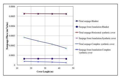
Figure 2. Effect of lengths of blanket, horizontal synthetic and complete on seepage flow
