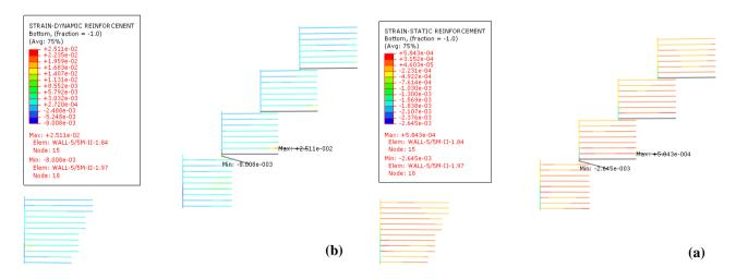
Figure 7. Strains of the reinforcements: (a) end of construction, (b) dynamic loading
