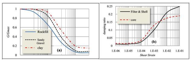
Fig 6. a) shear modulus curves of dam body materials, b) damping ratio curves of dam body materials
