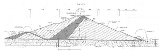
Figure 1: Cross section of initial dam
