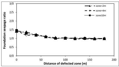
Figure 4. The graph of foundation seepage ratio versus defected zone location (X); the dam has height (H) of 20 m and foundation with permeability of  $1^{-2}$  m/s and different width of defected zone in upstream blanket
