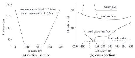
Figure 4. Breach sections of Banqiao reservoir
