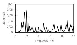
Figure 5-PSD spectrum of vertical component of Kobe near field motion
