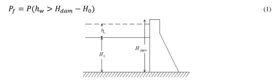
Figure 1. A view of dam height, initial height of water in dam reservoir and increasing water height due to the wind
