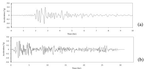
Figure 2. Time-acceleration diagram for: a-Coalinga earthquake (1983), b-El-Centro earthquake (1940)
