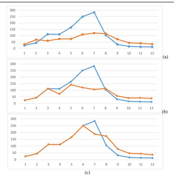
Figure 9. Long-lead forecast of inflow to the Seimarch reservoir generated at October 2013 (a) January 2014 (b), and March 2014 (c) (Red and Blue Lines demonstrate the forecast and observed values, respectively. The unit of the vertical axis is Million Cubic Meter)
