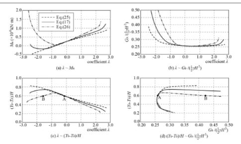
Fig. 9. The influences of  $\lambda$  on the unbalanced moment and the active earth pressure as well as its point of application for a given circular failure surface ( $\phi 0 = 54^{\circ}$ ,  $\Delta \phi = 11.6^{\circ}$ )
