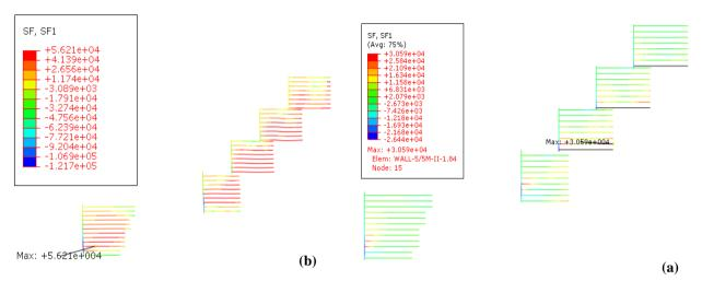
Figure 6. Distribution of maximum tensile forces at different heights in walls at: (a) end of construction, (b) dynamic loading
