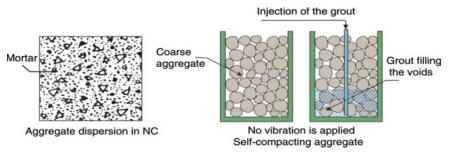
Figure 1. Theory of concreting
