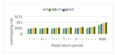
Figure 5. The effect of wind and flood return period changed on overtopping risk by considering uncertainty of water initial level
