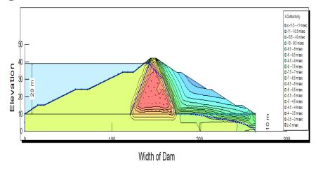
Figure 4: Hydraulic Conductivity at CH700 (Conductivity: 1.4628577e-007)
