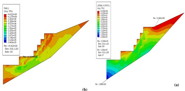
Figure 4. Distribution of lateral pressure: (a) end of construction, (b) dynamic loading
