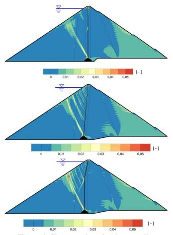
Figure 9. Shear strains after impounding
