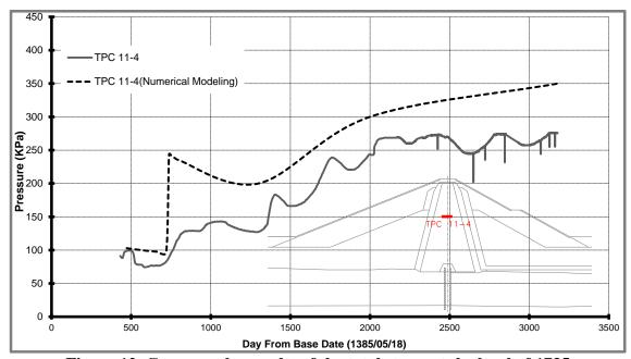
Figure 12. Compare the results of the total stress at the level of 1735
