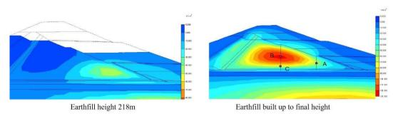
Figure 6: Example of estimated pore pressure during the construction phase
