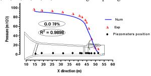
Figure 6. Average pressure variation along the conduit on the floor at 30% gate opening
