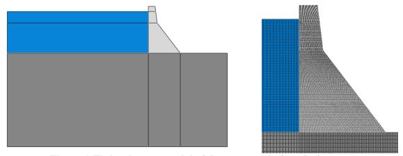
Figure 1-Finite element model of dam-reservoir-foundation system
