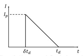
Figure 2. Abrupt wave inflow hydrograph
