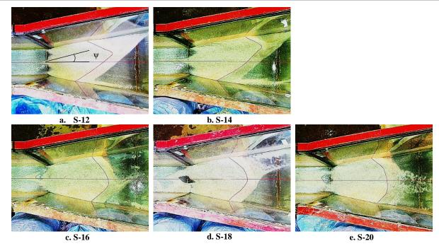
Figure 6. Delta direction in steady flow (Flow from left to right)
