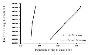
Fig4. The effect of cut off wall in dissipating the piezometric pressure
