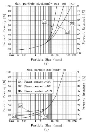
Figure 1. Gradation curve of testing materials a) Different maximum particle sizes b)
