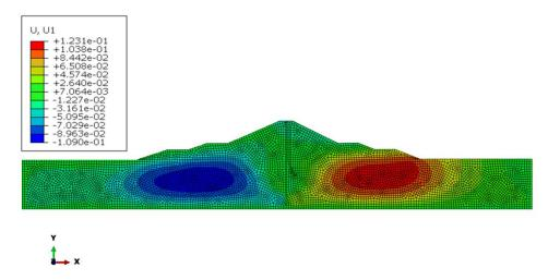
Figure 9. Total Horizontal Displacements at the End of Construction Stage Considering the Sealing Wall Implementation up to the Crest Level
