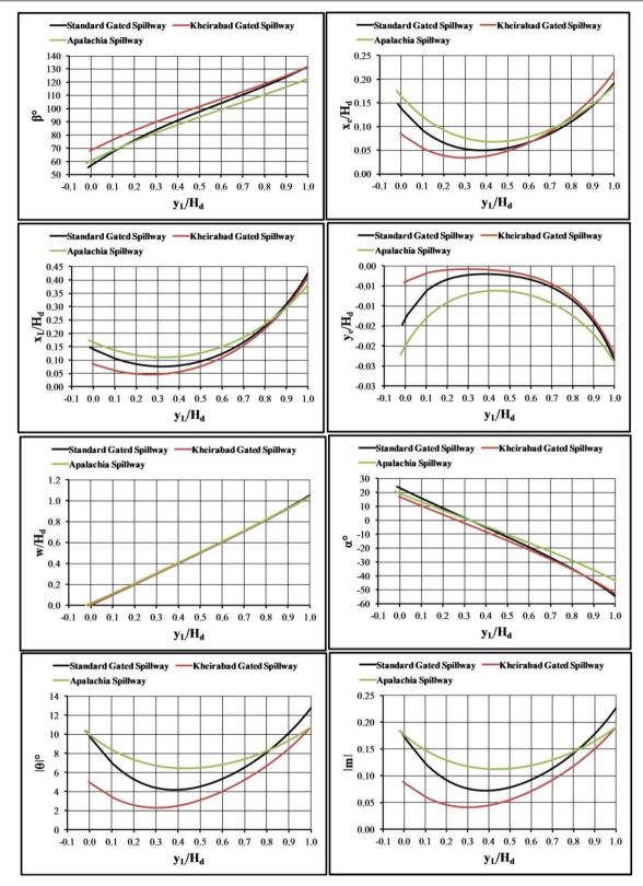
Figure (3)- Variation of  $\beta$ ,  $x_c/H_D$ ,  $x_L/H_d$ ,  $y_c/H_d$ ,  $w/H_d$ ,  $\alpha$ ,  $|\theta|$ , |m| with  $y_L/H_d$  using the new proposed method and for three gated spillways with the different downstream face
