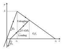
Figure 2. Softening curve of concrete under uniaxial cyclic loading
