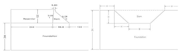
Figure 1. geometric characteristics of 2D Pine Flat dam section
