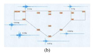
Figure 1. a) View of Karun III dam, b) Location of accelerometer installed on Karun III dam and upstream-downstream component of November 20, 2007 earthquake
