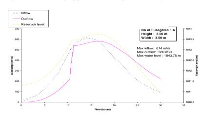
Figure 12: Dam equipped with fusegates for 10 years flood
