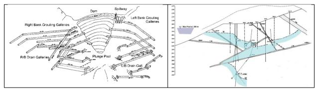
Figure 7: Thissavros dam, arrangement of drainage and grouting galleries and hydrogeological section of right abutment. Hatching represents groundwater.
