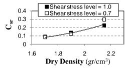
Figure 9. Coefficient of stress recovery (Csr) versus initial dry density
