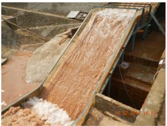
Figure 8. Lower chute and lower basin entry Q1,000
