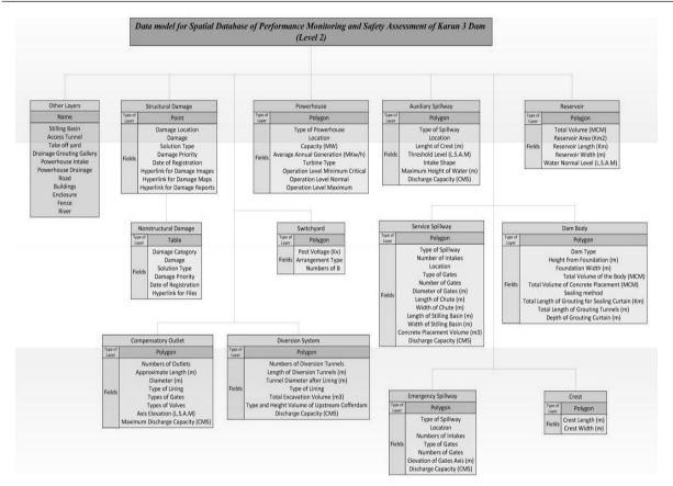
Figure 3- GIS data model (Level 2) - Karun 3 Dam [3]
