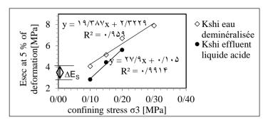
Figure 8. Variation of the secant modulus as a function of lateral stress
