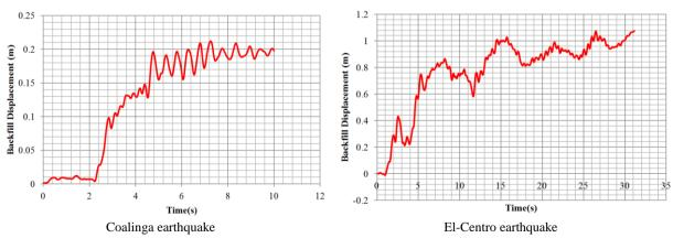
Figure 5. Horizontal displacements of walls
