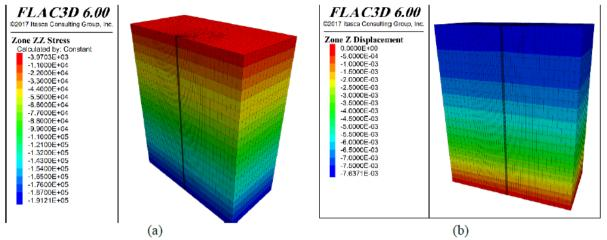
Fig 4- a) Stress contour, b) Displacement contour
