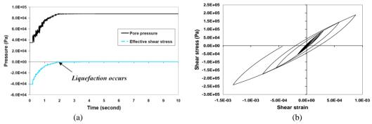
Figure 4. Simulation of cyclic simple shear test of one-zone sample in FLAC: (a) pore pressure generation and effective stress time histories during the dynamic loading, and (b) hyteresis loops
