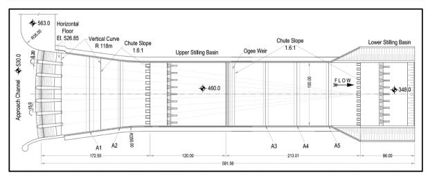
Figure 4. Plan of the double basin spillway
