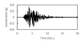
Figure 4-Vertical component of Kobe near field motion
