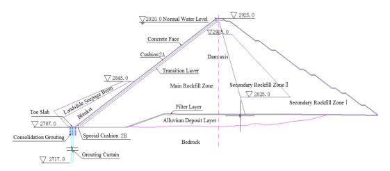
Figure 1. Cross section of the CFRD considered in the present study.
