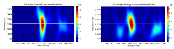
Figure 6- CWT of third motion and identifying first mode
