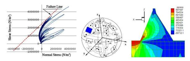
Figure 8 a) stress path on plane no. 8, b) its direction on sphere, and c) initial P.W.P.
