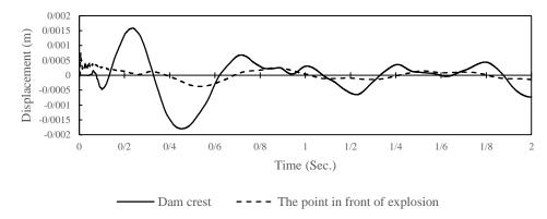
Figure8-time history of displacement for the case of explosion near to mid height of the dam
