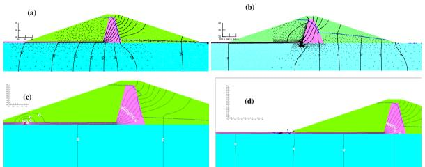
Figure 2. The flow pattern from seepage analysis of dam with height of 20m and foundation permeability of K=10<sup>-4</sup> m/s: a) intact impervious blanket, b) defected zone next to clay core connection point (X=0), c) defected zone inside the dam body (X=40 m), d) defected zone outside of dam body (X=60 m)
