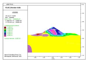
Fig 12. Horizontal displacement contours (m)
