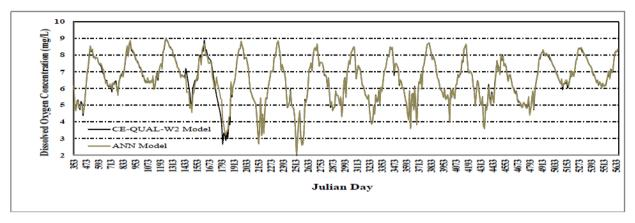
Figure 3. Comparison the performance of DO neural network model with CE-QUAL-W2
