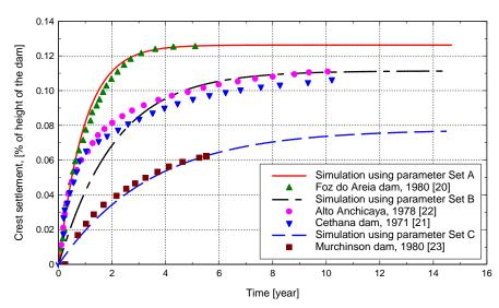
Figure 6. Evolution of crest settlements within a 15 year period after water impounding:
