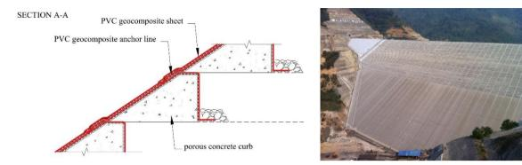
Figure 6. Face anchorage with PVC anchor strips embedded in curbs: concept and staged installation at Nam Ou VI 88 m high rockfill dam in Lao PDR
