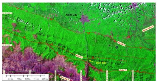
Figure 1. Illustration of Major Faults on LANDSAT Image
