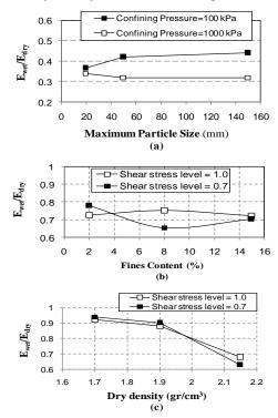
Fig. 11 Ratio of the saturated to dry elasticity modulus of the material  $(E_{wet}/E_{dry})$ , a) versus material maximum particle size, b) versus fines content, c) versus initial dry density
