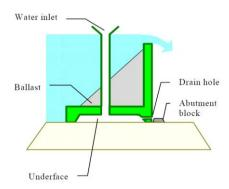
Figure 3: water spills over the Fusegate
