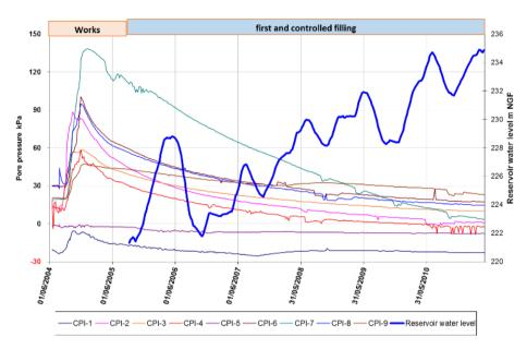
Figure 13: Pore pressure after works and during first and controlled filling
