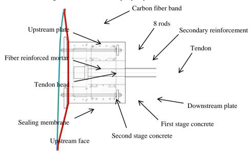
Figure 8. Carbon fiber net anchoring device
