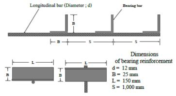
Figure 1 (a) Typical configuration of the bearing reinforcement
