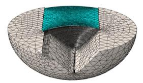
Figure3-finite element model of damreservoir-foundation of Karun IV
