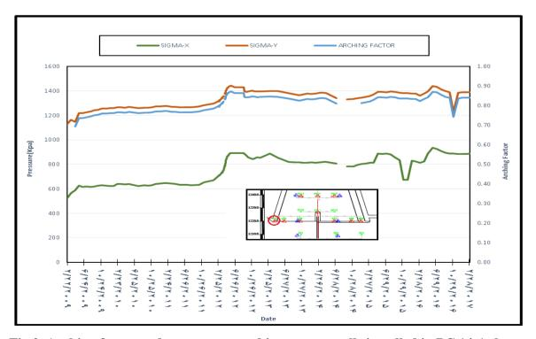
Fig 2. Arching factor and stress measured in pressure cells installed in PC 14-1 cluster
