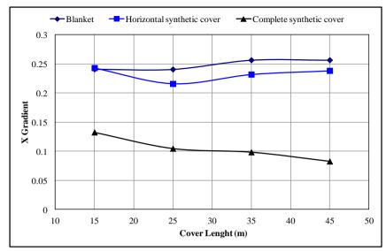
Figure 3. Effect of lengths of blanket, horizontal synthetic and complete on exit gradient
