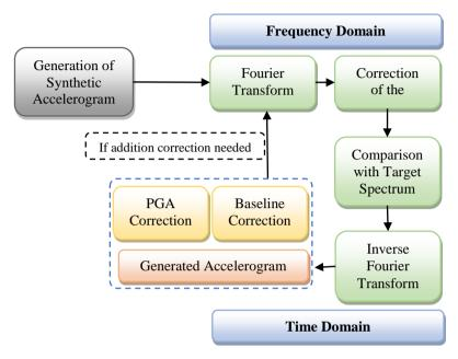
Figure 1. Algorithm of generating synthetic ground motion
