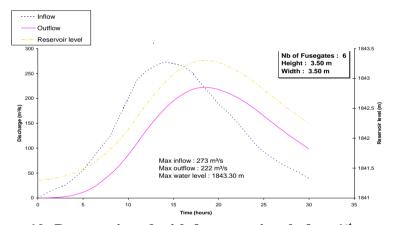
Figure 10: Dam equipped with fusegates just before 1st reversing
