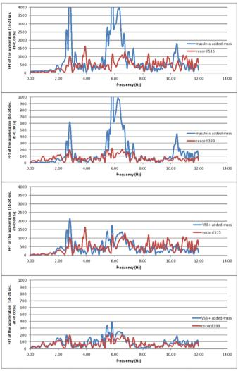
Figure 3comparison of the FFT of the horizontal acceleration, recorded vs computed at the crest (top) and bottom of the dam (bottom) for Massless / added-mass model (left) and VSB / potential fluid model (right),
