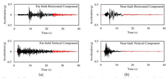
Figure 2: Truncated ground motion time histories (a) far-field; (b) near-fault
