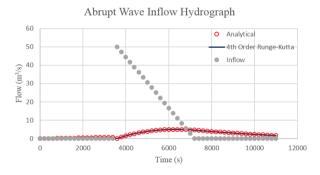
Figure 6. The outflow of abrupt wave inflow hydrograph
