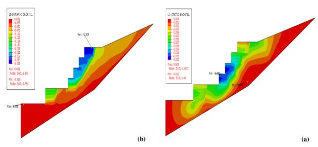
Figure 5. Horizontal displacement of backfill soil: (a) end of construction, (b) dynamic loading
