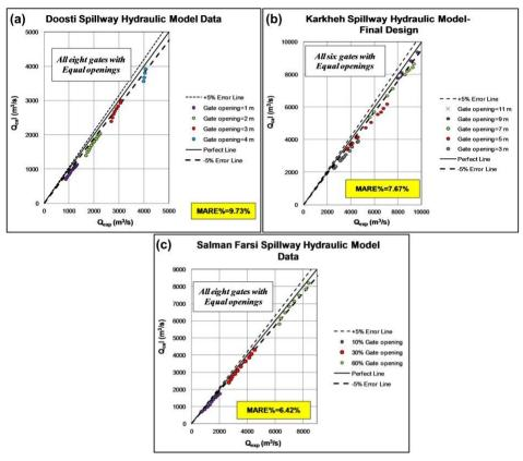
Figure (8)- Effect of downstream weir face on the discharge estimation of gated spillway using USACE (1977)'s method
