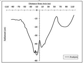
Fig 14. Settlements profile along pipes of diversion system (cm)
