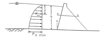
Figure 4. Distribution of hydrodynamic pressure on Dam [1]
