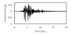
Figure 2-Horizontal component of Kobe near field motion
