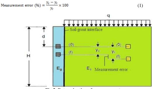
Fig 5- Determination of measurement error
