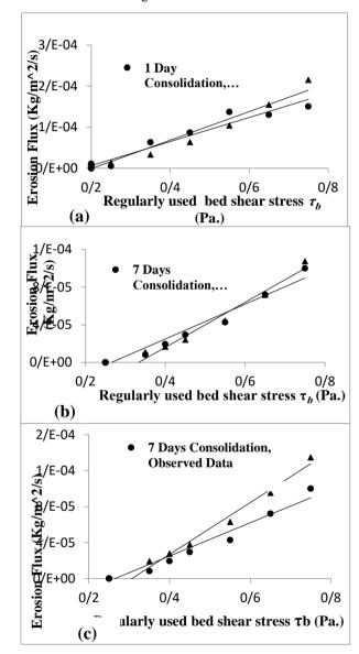
Fig.1 Comparison between experimental data of resuspension flux and formulation results
