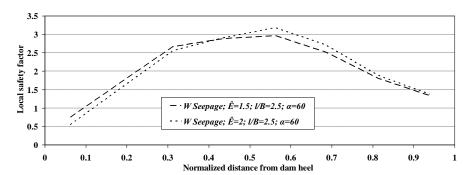
Figure 5. Local sliding safety factor along the dam base for the critical models while seepage is included.
