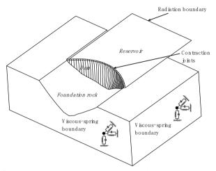
Figure 1. Sketch of the arch dam-water-foundation rock system
