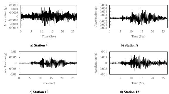
Figure 2- Recorded accelerations. A) station 4. B) station 8. C) station 10. D) station 12.
