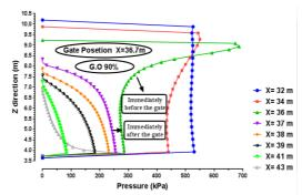
Figure 14. The profile of flow velocity distribution in vertical sections of outlet conduit in vicinity of service gate for 90% gate opening
