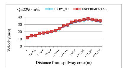
Figure 5- The comparison between numerical and experimental velocity for (2290 m<sup>3</sup>/s)
