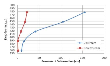
Figure 6. Results of permanent deformation in different elevation- Haraz Dam
