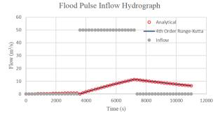
Figure 7. The outflow of flood pulse inflow hydrograph
