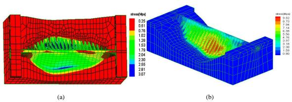
Figure 5 Dam combined stress analysis, a) before and b) after earthquake
