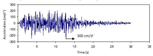
Figure 2. Synthetic acceleration-time history of OBE plot for input motions used in the dynamic analysis of Bebekli dam.
