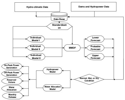
Figure 2. Conceptual model of FARDA system
