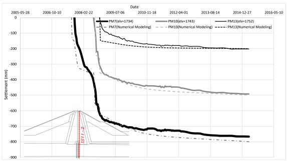
Figure 14. Comparison of the results of settlement in core at the levels of 1734, 1743, and 1752
