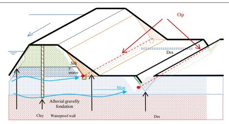
Figure 3: 3D view of the canal embankment after its rehabilitation
