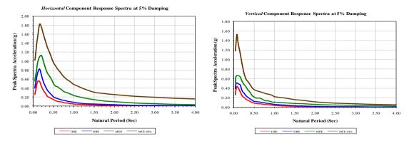
Figure 2. Acceleration Response Spectra for the dam site
