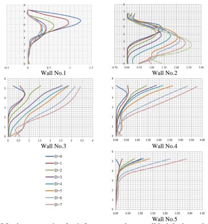
Figure 10. Maximum strain of reinforcement along wall height in each stage of multitiered soil walls after El-Centro earthquake
