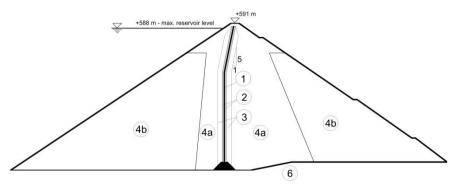
Figure 3. Design with partially inclined core
