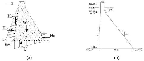
Figure 1. (a) Schematic representation of dominant static loadings applied on a gravity dam's section; (b) the tallest non-over-flow monolith of Pine Flat dam (all dimensions are in meter).
