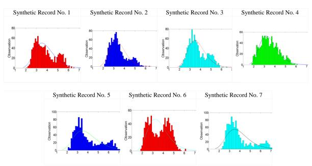
Figure 4. The histograms of the maximum tensile strees obtained by LHS under synthetic ground motion excitation. The horizontal and vertical axes are the tensile stress (MPa) and number of observation, respectively.
