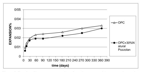
Figure 8. Results of long term expansion of specimens containing natural pozzolan
