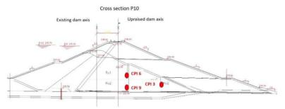
Figure 8: Location cross section of monitoring points
