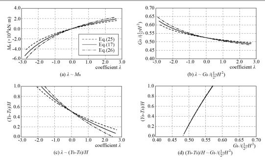
Fig. 8. The influences of  $\lambda$  on the unbalanced moment and the active earth pressure as well as its point of application for a given circular failure surface (c = 0,  $\phi$  = 35°)
