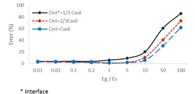
Fig.8 Error percentage of measurement with different interface cohesion for different (Eg/Es) ratios for medium soil
