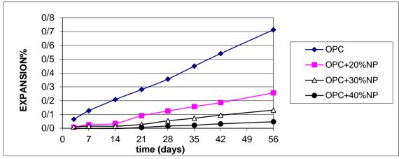
Figure 7. Results of accelerated mortar bar tests containing natural pozzolan
