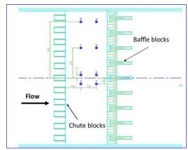
Figure 11. Transducer locations in the upper basin for one test configuration
