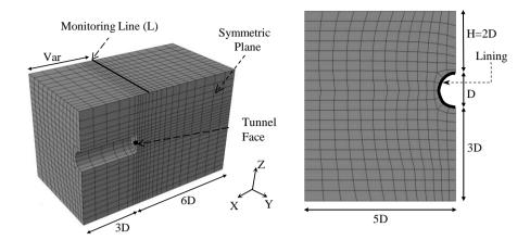
Figure 3. Finite element model of the simulated tunnel
