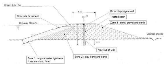
Figure 2: Cross section of the canal embankment before its rehabilitation 3
