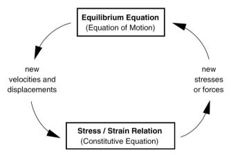
Figure 1. Basic explicit calculation cycle [4].
