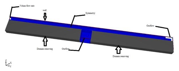
Figure 3. Boundary conditions of rectangular side weir in circular channel in numerical model
