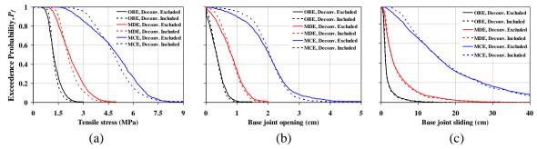
Figure 6. Effects of the earthquake deconvolution process on the EP curves for (a) overstressing, (b) base joint opening, and (c) base joint sliding performance functions
