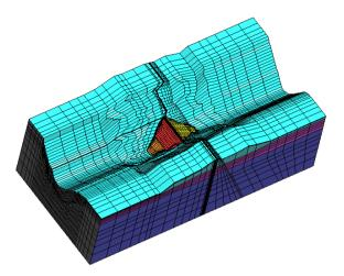
Figure 2. Finite element mesh of dam and foundation.
