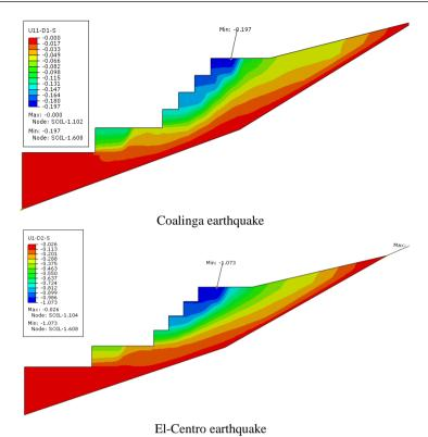
Figure 8. Contour of horizontal displacements of walls
