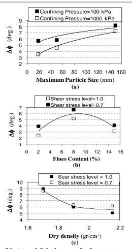
Figure 10. Reduction of internal friction angle due to saturation ( $\Box \Box c$ ), a) versus material maximum particle size, b) versus fines content, c) versus initial dry density
