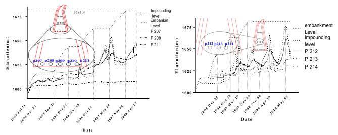
Fig2. Second level piezometric pressure results from piezometers of cross section 2
