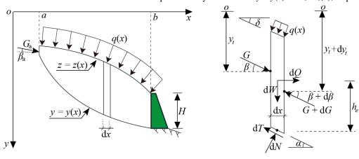
(a) The slope-retaining wall system
