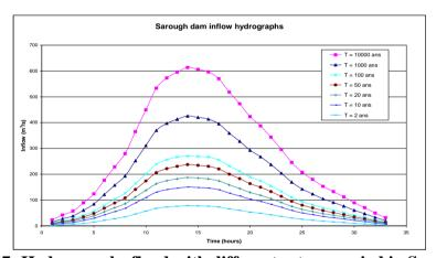
Figure 7: Hydro graphs flood with different return period in Sarough Dam
