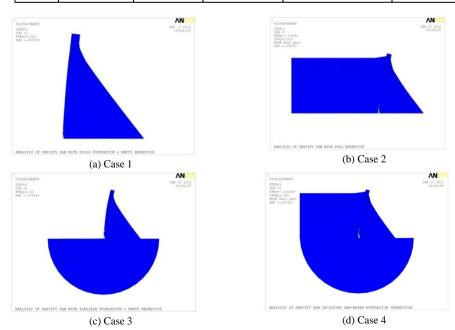
Figiure 3. The first mode shape of the dam for different Cases
