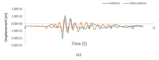
Figure 4. Graph of comparison of displacement time histories in stream direction at central crest point for Uniform and Non-uniform records at three performance level a) DBE, b) MDE and c) MCE
