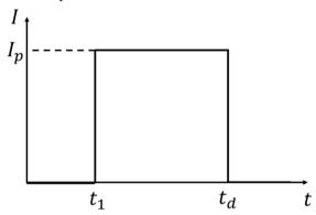
Figure 3. Flood pulse inflow hydrograph
