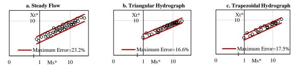
Figure 8. Length of delta versus mass of sediment
