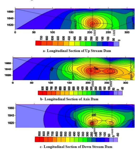
Fig 8. Settlement counters of longitudinal sections of dam at service time
