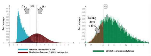
Figure 8. Dasht-e-Palang dam probabilistic analysis results
