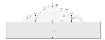
Figure.3. optimization of cross section of an earth dam
