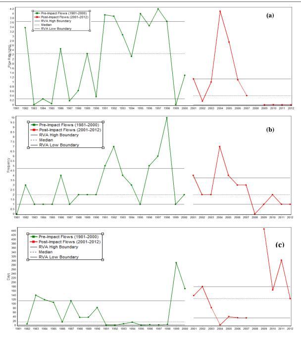
Figure 9 . Comparison of the (a) Mmagnitude, (b) Frequency, and (c) Duration of extreme low flows before (green line) and after (red line) operation of the Hasanlu reservoir.
