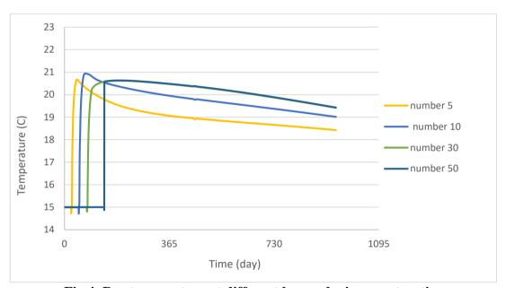
Fig.4. Rcc temperature at different layers during construction
