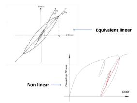
Figure 2. Comparison of equivalent linear behavior and actual behavior of materials in cyclic loading
