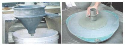
Figure 2. Flow cone and flow meter setup
