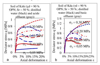
Figure 7. Diagram deviator stress - axial deformation (UU test)
