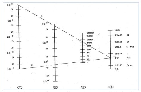
Figure 1: Determine The drop of pressure in rods (Amoco, 1994), (rods of metal and for length 10 m in comments taken made); 1-drop the pressure, dp (in MPa), 2-viscosity stream,  $\nu$  (Cm/S), 3-Discharge, Q (l/min), 4-diameter of pipe, D (mm, in)
