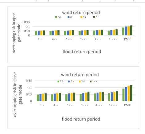
Figure 8. The comparison of overtopping risk due to flood and wind for close and open bottom outlet mode
