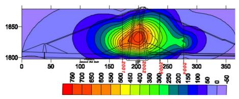
Fig7. Settlement counters of cross section 2 in service time
