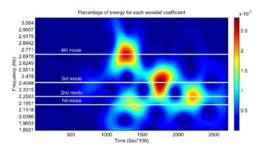
Figure 4- CWT of first motions and identified frequencies
