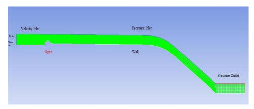
Figure 2: The calculation domain and boundary conditions.
