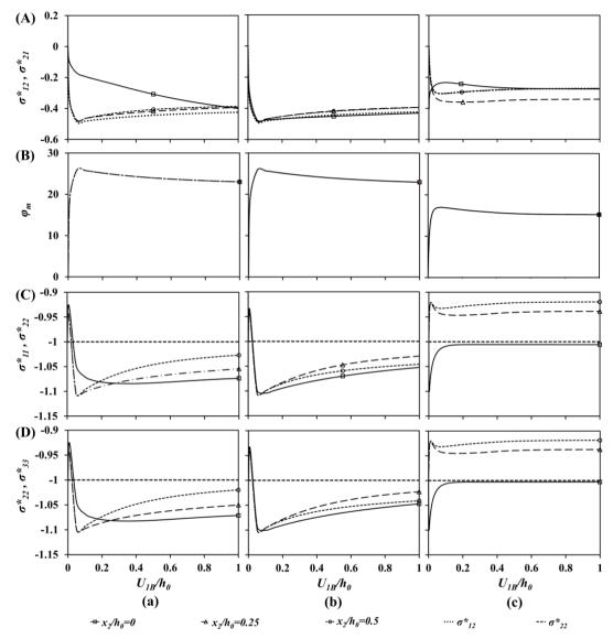
Figure 4. Evolution of (A)  $\sigma_{12}^*$ ,  $\sigma_{21}^*$ , (B)  $\varphi_m$ , (C)  $\sigma_{11}^*$ ,  $\sigma_{22}^*$  and (D)  $\sigma_{22}^*$ ,  $\sigma_{33}^*$  at different  $x_2/h_0$  for: (a) Case (1):  $f_T = 0$  and  $f_B = 0.0001$ , (b) Case (2):  $f_T = 0$  and  $f_B = 0.01$  and (c) Case (3):  $f_T = 0$  and  $f_B = 0.5$
