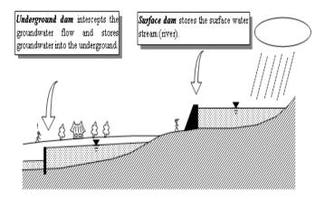
Figure 5. Scheme of surface dam and underground dam [14].
