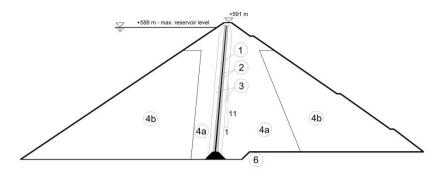
Figure 2. Design with inclined core
