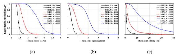
Figure 5. EP curves of the three sets of samples under increasing ground excitation intensities for: (a) overstressing, (b) base joint opening, and (c) base joint sliding performance functions.
