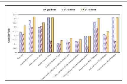
Figure 7. Comparison the combined effect of blanket, cutoff wall and synthetic cover on content of exit gradient
