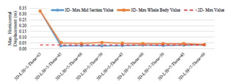
Figure 8- Comparison of Max Horizontal Displacement Value at Different Locations of Dam Body for 3D and 2D Analysis under PGA=0.3g Earthquake
