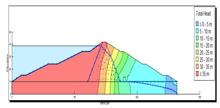
Figure 2: Total head variation at Ch.700 m (Total head :39m)
