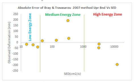
Figure 3. The absoluteerrors of the upper bound values of Bray and Travasarou 2007 coupled-based method (the designee method), for estimating max deviatoric deformations versus SED of the Group 1 case studies
