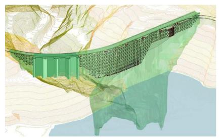
Figure 7. The carbon fiber net seen from upstream
