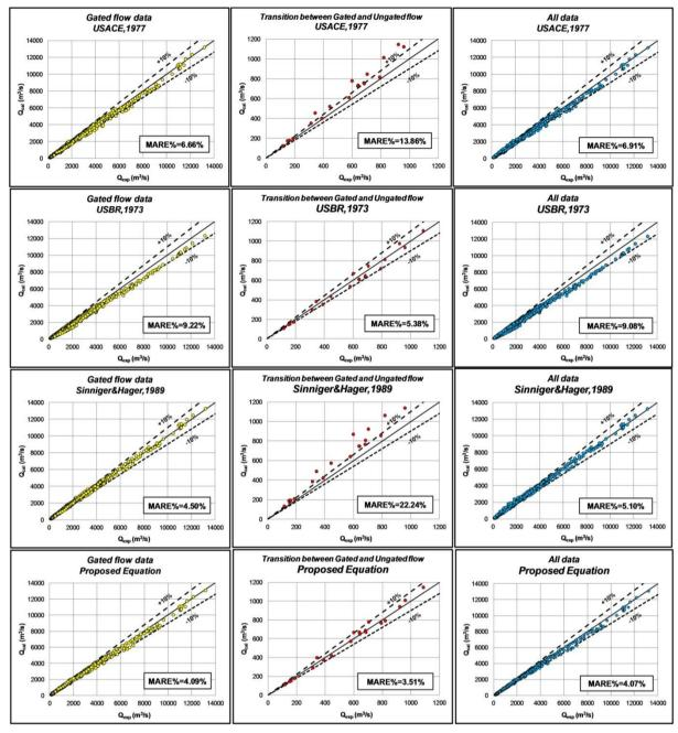
Figure (7)- Evaluation of different methods for the discharge estimation of gated spillways using Gated and Transition flow data
