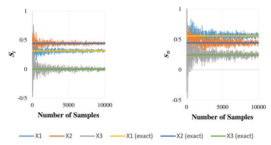
Figure 2. Verification of implemented VBSA (Sobol' indices) tested for equation 4.
