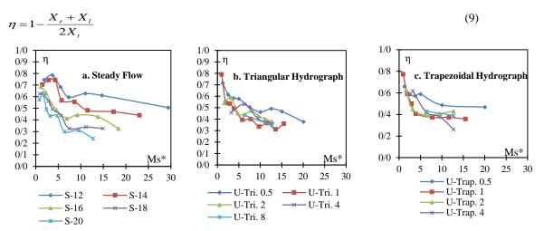
Figure 9. Variations of the convexity parameter versus sediment mass
