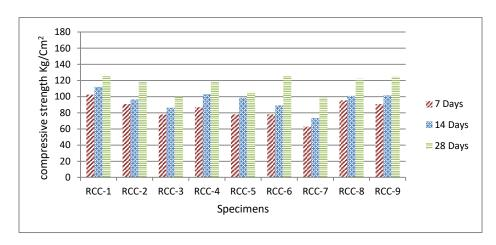
Figure 6. 7, 14, 28-days compressive strength results
