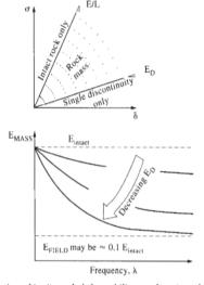
The modulus of deformation of a rock mass containing a discontinuity set.
