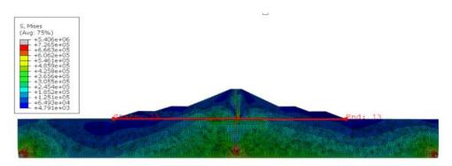
Figure 6. select section for check the maximum stress in the cut-off wall proposed 100 cm
