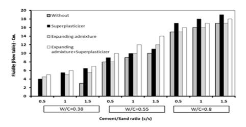
Figure 4. Flow table test results
