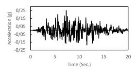
Figure 6-Horizontal component of Kobe far field motion
