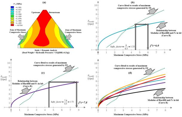
Figure 1. Modulus of deformation vs. compressive strength
