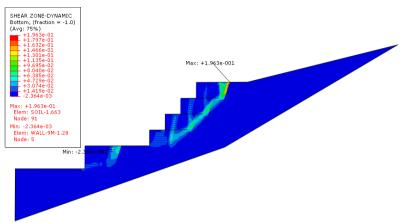
Figure 8. Shear zone at end of dynamic loading
