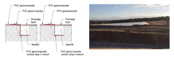
Figure 5. Face anchorage with PVC anchor strips embedded in trenches: concept and installation at Bulga new earthfill dam, Australia
