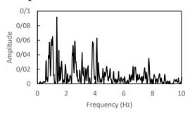
Figure 9-PSD spectrum of vertical component of Kobe far field motion
