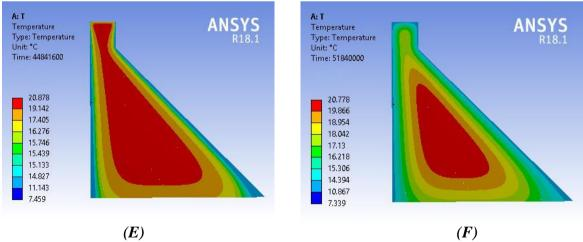
Fig.7. Temperature in °C during construction on 27.01.2009 (E) and 16.05.2009 (F)
