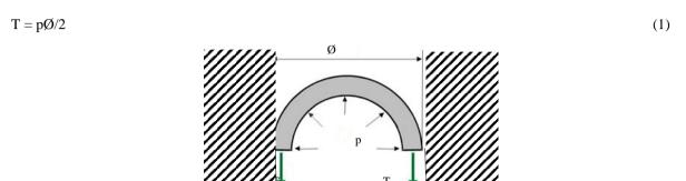
Figure 3. Typical cross section (not to scale) illustrating forces applying on free edges of the bladders.
