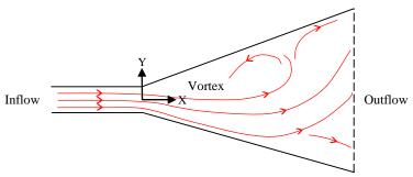
Figure 3. Schematic diagram of flow deviation and vortex formation in the reservoir
