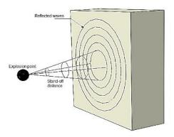
Figure 1- Schematic of air blast
