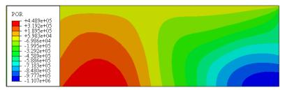
Figure 16-Contours of hydrodynamic pressure in 5.51 second due to Kobe near field motion
