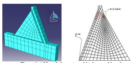
Figure 6 a) Maped elements and b) damaged locations
