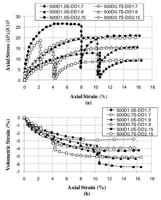
Figure 5. a) Axial stress-axial strain b) volumetric strain-axial strain behavior of series C tests, Effect of initial dry density
