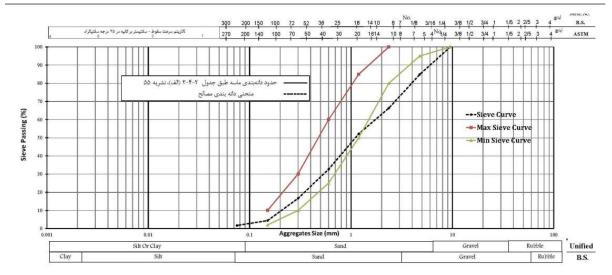
Figure 2. Particle-Size Analysis of Fine-aggregates (0-6 mm)
