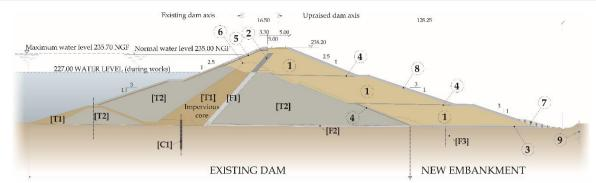
Figure 4: Upraising dam cross section
