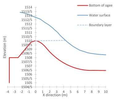
Figure 8: Flow pattern for Q=1006 m3/s
