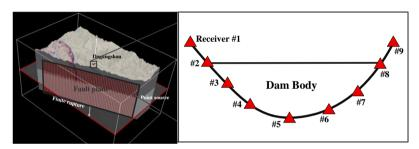
Figure 8. Three dimensional numerical model of Dagangshan dam site
