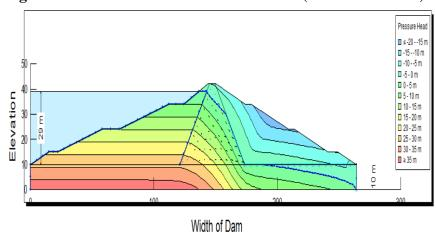
Figure 3: Pressure head variation at Ch.700 m (Total head :29m)
