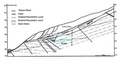
Figure 12: Geological and hydrogeological conditions at Cairnmuir Slide. Mainly the drainage of the sub-basal confined aquifer stabilized the slide. Hatching marks groundwater below main failure plane.
