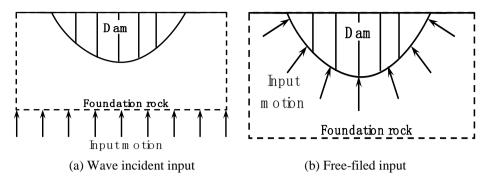
Figure 3. Earthquake input mechanism
