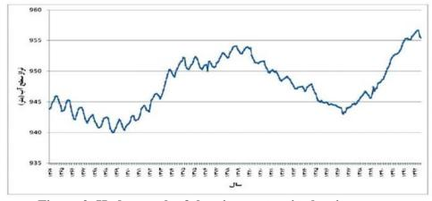
Figure 2. Hydrograph of the piezometers in the city center.
