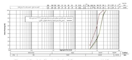
Figure 1. Particle-Size Analysis of Coarse-aggregates (6-25 mm)
