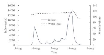
Figure 5. Inflow and water level variation of Banqiao reservoir during "75.8" flood
