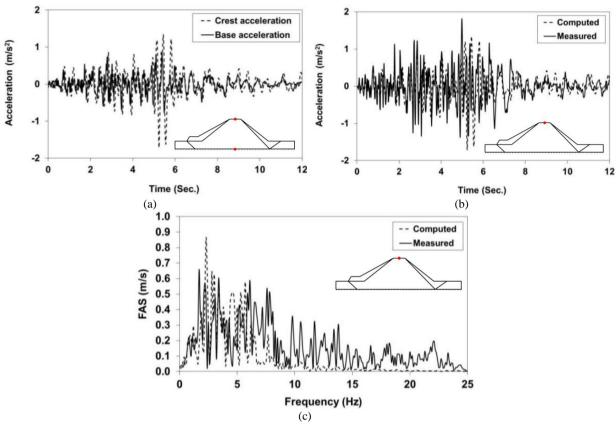
Figure 12. Comparison between computed and measured values of LV dam in vertical direction at: (a) crest and base, (b) crest acceleration time histories, and (c) Fourier amplitude spectrums
