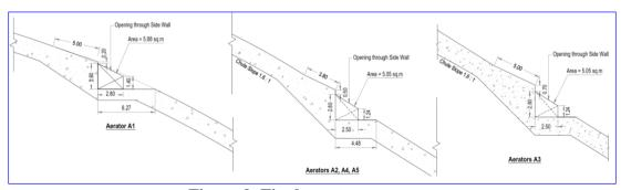
Figure 9. Final aerator geometry
