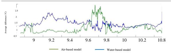
Figure 7: Temperature difference between the water-based model and the optic fiber temperature (blue line) and between the air-based model and the optic fiber data (green line)
