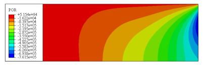
Figure 18-Contours of hydrodynamic pressure in 13.63 second due to Kobe far field motion
