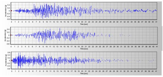
Figure 6. Khorgu scaled accelerograms components in the MCL
