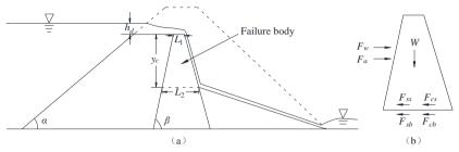
Figure 8. Shear failure of clay core
