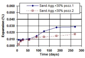
Figure 5. Expansion of prisms made with sand
