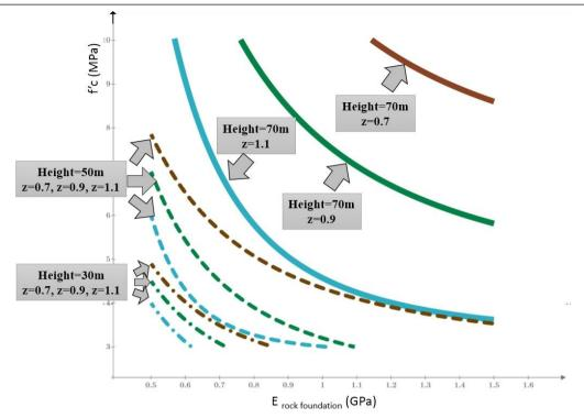
Figure 9. Relationship between modulus of foundation and optimum f'c of Hardfill
