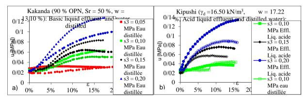
Figure 7. Diagram pore pressure – axial deformation in CU
