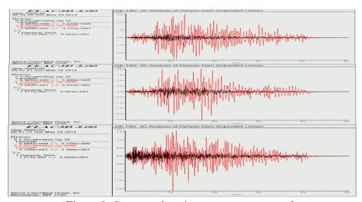
Figure 9. Crest acceleration components records
