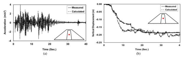
Figure 8. Measured versus calculated results of centrifuge modeling: (a) acceleration, and (b) displacement time histories at the middle of dam height
