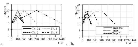
Figure 2. Different hydrographs used in unsteady experiments: (a) triangular hydrographs and (b) trapezoidal hydrographs
