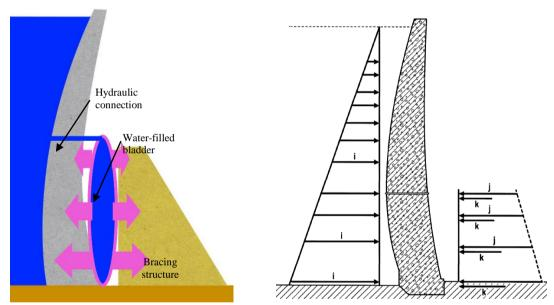
Figure 1 (left). Schematic cut-away drawing illustrating the concept.
