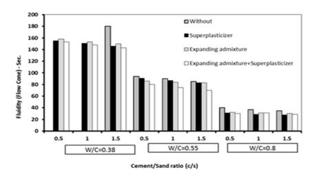
Figure 3. Flow cone test results
