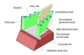
Figure 2: Typical 3D view of a Fusegate
