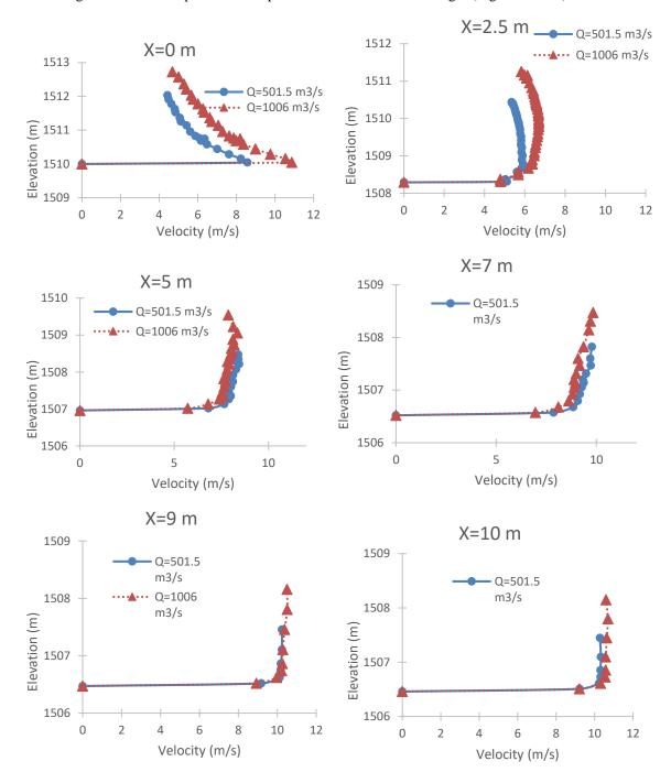
Figure 5:Comparison of velocity profile between discharges of 501.5 m3/s and 1006 m3/s in six sections (x=0, 2.5, 5, 7, 9 10)
