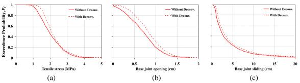
Figure 7. Comparison of the EP curves of the 1000-sample set under the MDE with and without deconvolution: (a) overstressing, (b) base joint opening, and (c) base joint sliding
