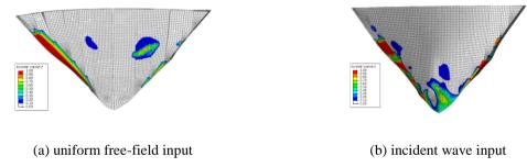
Figure 6. Dam damage with different earthquake input mechanisms
