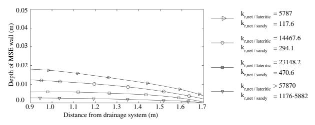
Figure 7 Variation in phreatic surface in the protected zone for various ratios between the hydraulic conductivity of the geonet and that of soil
