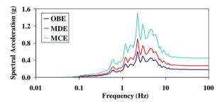
Figure 3. Response spectra of the selected earthquake ground motions
