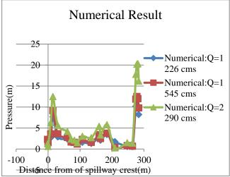
Figure 4-a) The comparison between numerical and experimental static pressure for discharge (1226 m<sup>3</sup>/s)
