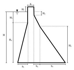
Figure 1. Geometrical model of concrete gravity dam
