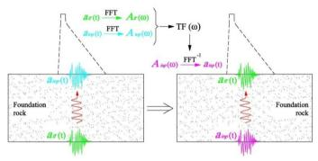
Figure 1. Schematic representation of the deconvolution process
