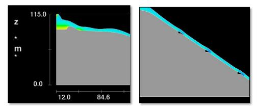
a) Pressure changes near aeration chute b) Pressure changes on ogee spillway crest Figure 4- The manner of changes in the static pressure on the spillway and chute of Azad dam (for maximum discharge)
