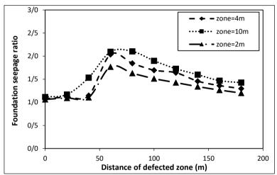
Figure 5. The graph of foundation seepage ratio versus defected zone location (X); the dam has height (H) of 20 m and foundation with permeability of  $1^{-2}$  m/s and different width of defected zone in upstream blanket
