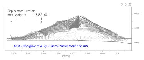
Figure 12. Displacement vectors of 2D analysis
