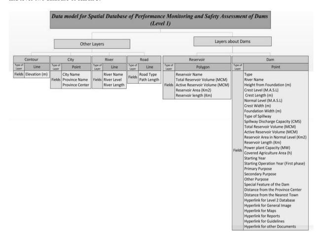
Figure 2- GIS data model (Level 1) [3]
