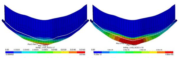
Figure 3 opening of the joint elements (left) and uplift propagation (right) on the dam/foundation and abutment/foundation interface (view from the top).
