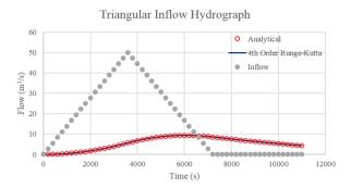
Figure 5. The outflow of triangular inflow hydrograph
