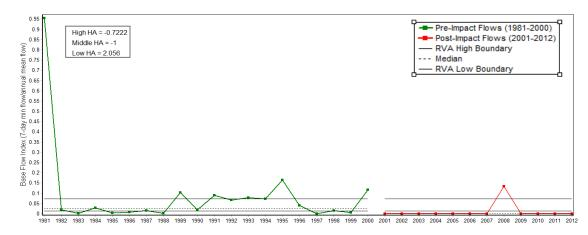
Figure 8. Comparison of the base-flow Index before (green line) and after (red line) the dam operation.
