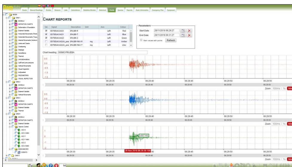
Figure 2: Graphical visualization of accelerometer data in DAMDATA
