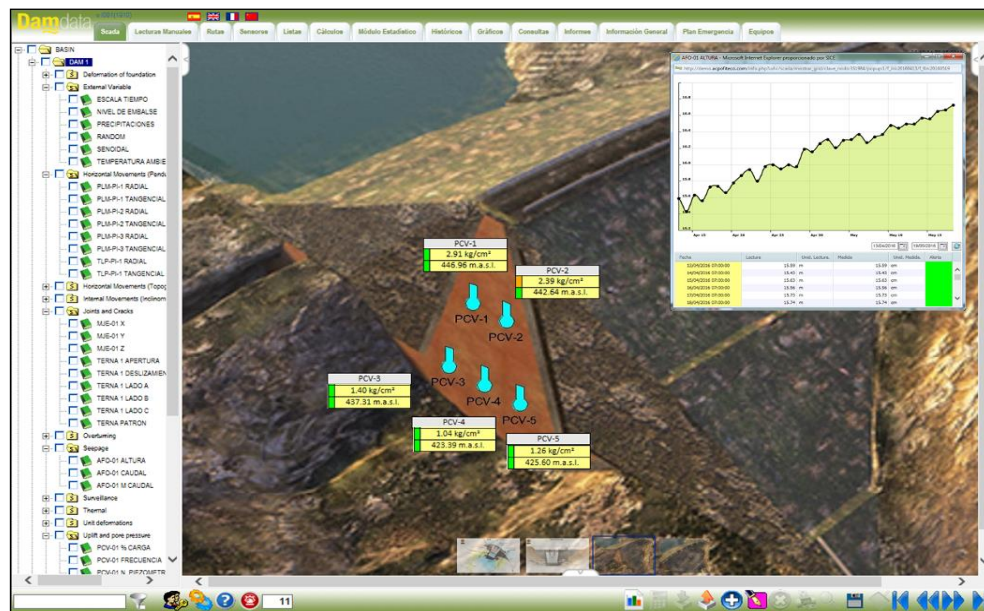
Figure 5. SCADA visualization of an embankment dam
