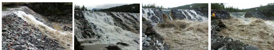
Figure 1. Large scale model test of moraine core rockfill dam due to overtopping failure
