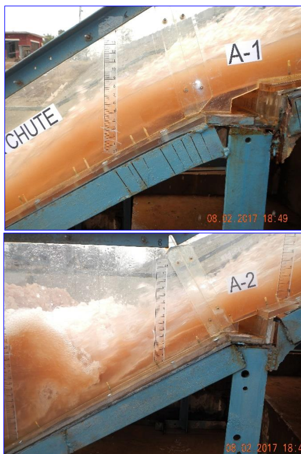
Figure 10. Nappe profiles at aerators 1 & 2
