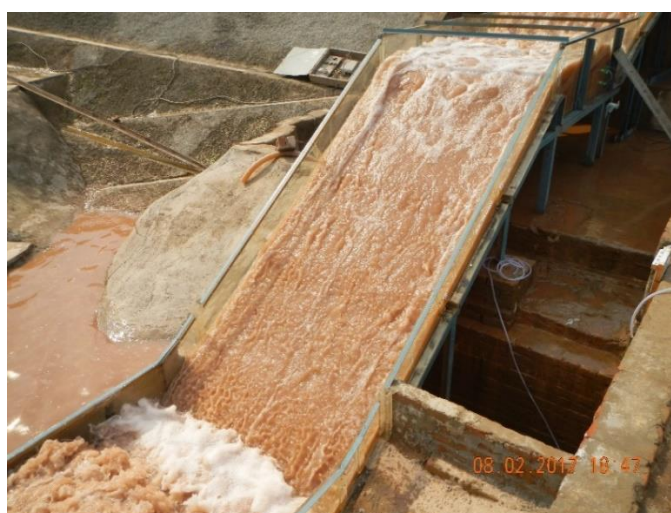
Figure 8. Lower chute and lower basin entry Q1,000
