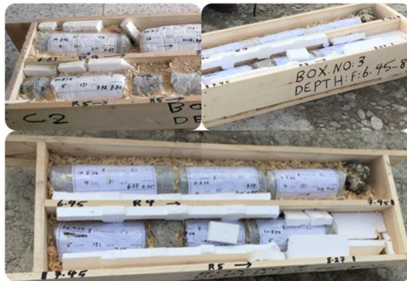
Figure 4. Core samples of Kahir dam
