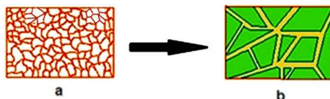
Figure 1 (a) Real aggregation of particles; (b) 2D representation of aggregation of artificial polyhedron
