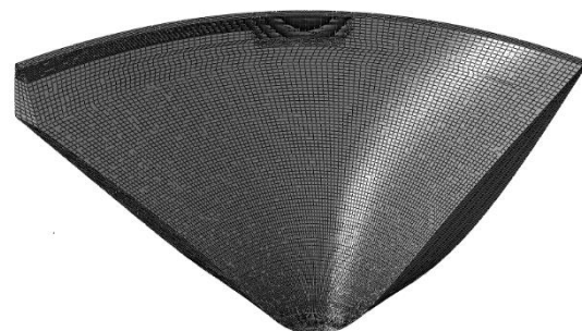
Figure4-finite element model of Karun IV dam for the case of explosion near to dam crest
