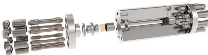
Figure 1: Exploded assembly drawing of the 30 mL reactor.
