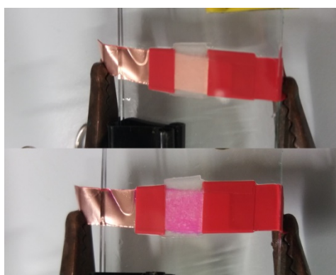
Fig 2: ECD that uses pH dye phenolphthalein in bleached (top) and tinted (bottom) state
