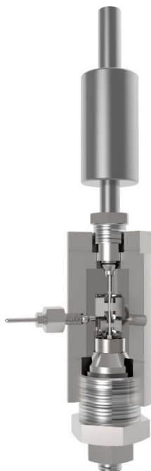
Figure 2: Assembled 100 mL autoclave with stirrer.
