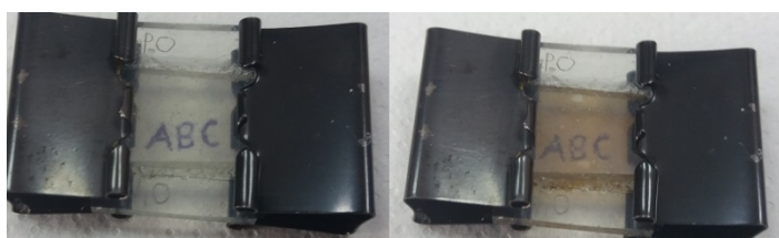
Fig 1: ECD that uses electrodeposition of PbO in bleached (left) and tinted (right) state
