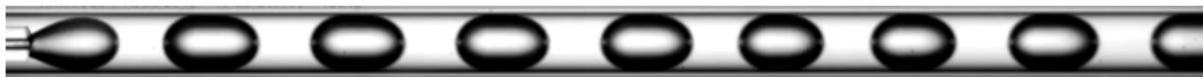
Fig 3. P = 20 MPa; T=308 K; V_{CO_2}= 0.02 mL.min -1 ; V_{H_2O}= 0.02 mL.min -1 in a 530 \mu m capillary.
