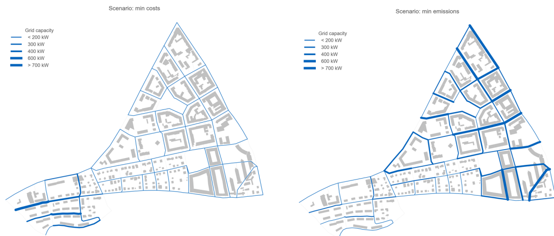
Figure 3: Electricity distribution grid capacity in the "minimum cost" scenario (left) and "minimum emissions" scenario (right)
