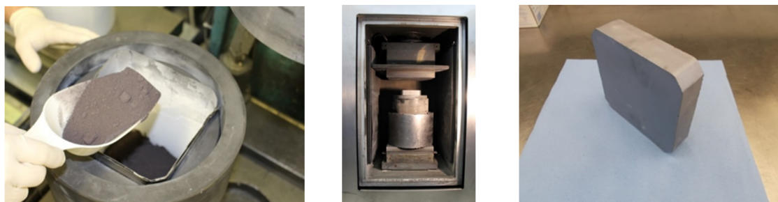
Figure 2: From left to right: (1) filling of the pressing mold with doped Si powder (2) setup of hot pressing (3) hot pressed Si ingot 156 mm x 156 mm x 40 mm (Photo: Peter Biermayr and Erich Neubauer)
