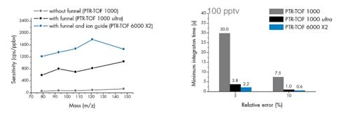
Figure 2: Comparison of measured sensitivities for different instrument types (left) and the calculated minimum integration times to reach a relative error of 5 and 10%, respectively (right).
