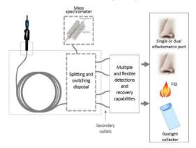
Figure 1: Schematic configuration of the InnOscent-GC device (patent pending) [3]
