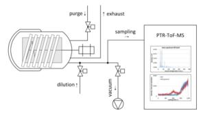
Figure 1: Schematics of the coupling of the PTR-ToF-MS to the reaction vessel for on-line PTR-ToF-MS analysis of the exhaust gas during roasting under controlled atmosphere.
