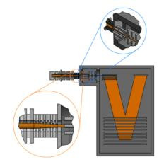
Figure 1: Schematic view of the novel PTR-TOF 6000 X2 equipped with an ion funnel (insert bottom left) and hexapole ion guide (insert top right).
