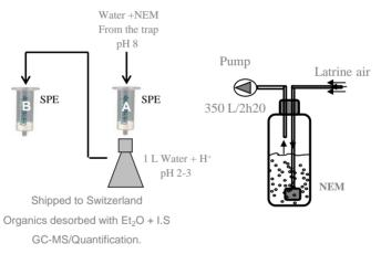
Figure 2: Schematic analysis of toilet headspace and quantification of  $H_2S$  and  $CH_3SH$  in addition to p-cresol, indole and butyric acid.
