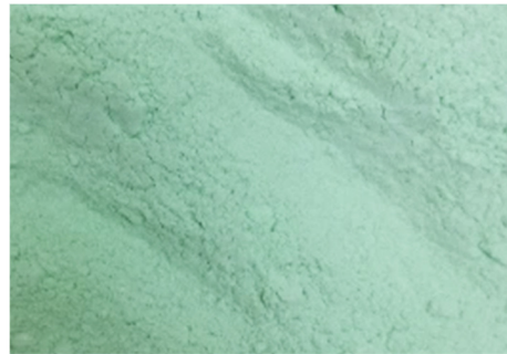
Fig. 2: Ni/MgO catalyst after impregnation
