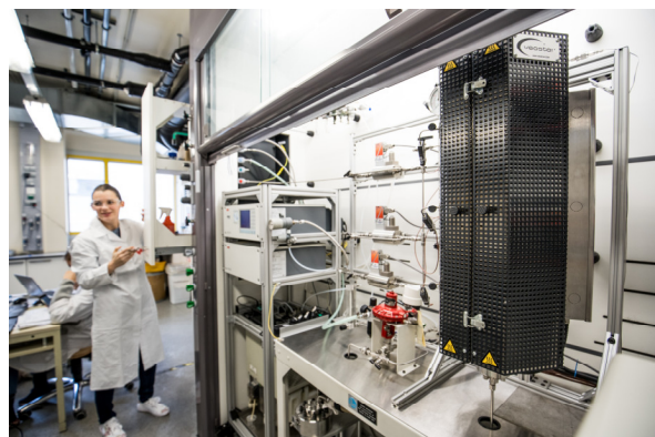
Fig. 3: Setup of the tubular reactor from parr industries
