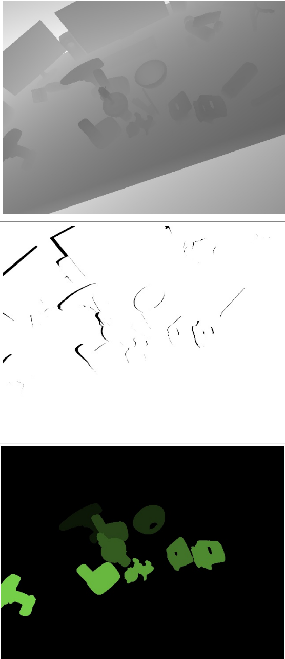
Figure 3. Synthetic depth image (top), visibility mask (middle) and pixel level class correspondence (bottom).
