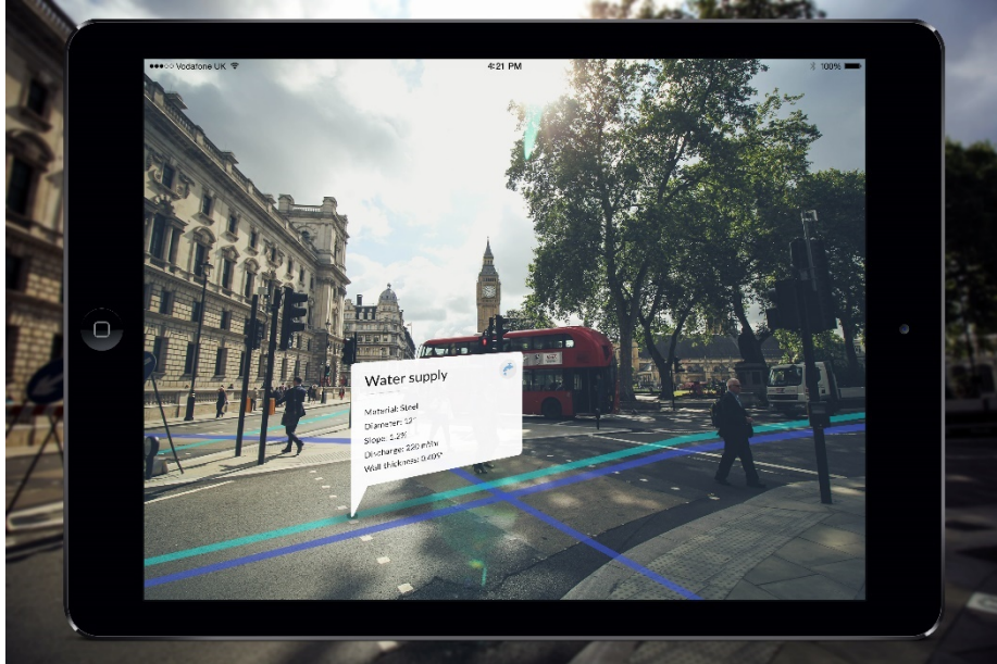
Fig. 9. Concept design of a prototype app for AR visualization of buried assets and the attribution of each individual physical item
