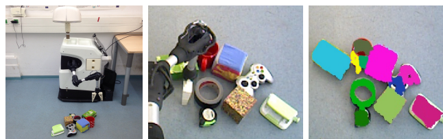
Fig. 1: Segmenting a cluttered scene with interaction. Left: Robot observing the scene. Middle: Robot inducing object motion. Right: Segmentation after interaction. Moved object (top left in blue) is correctly segmented.
