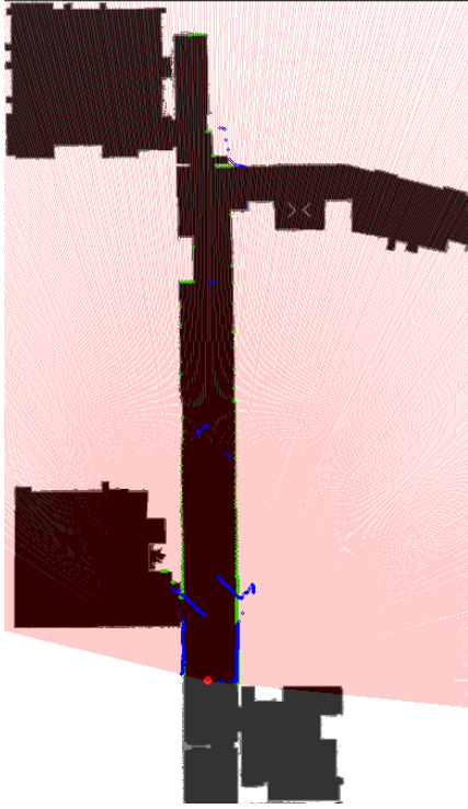
Fig. 2: Map of the office environment used for conducting the experiments together with a laser scan at time k .
