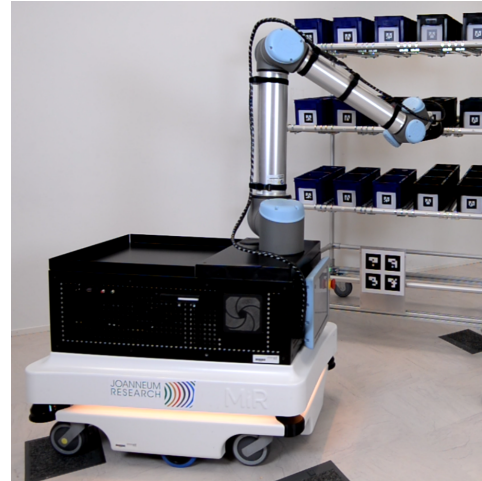
Fig. 1. Mobile manipulator (compilation of an UR10 and MiR100) solving an assembly task in a prototype industrial application
