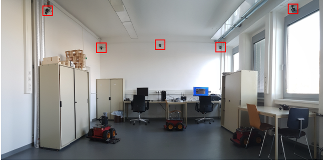
Fig. 7: Case studies laboratory, IR-cameras indicated in red.
