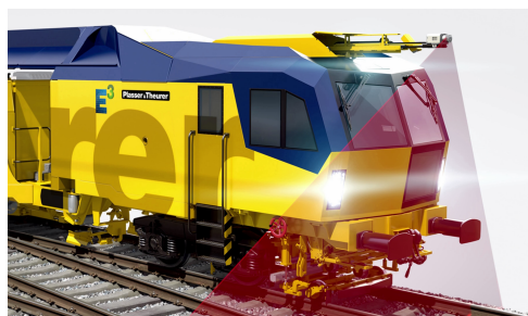
Fig. 1. Tamping machine with a roof-mounted 3D laser scanner.
