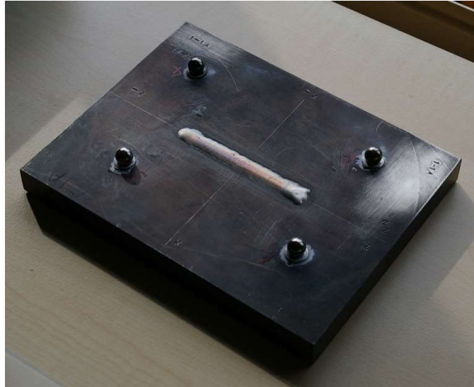
Fig. 2 Completed TG4 specimen prior to neutron diffraction measurements
