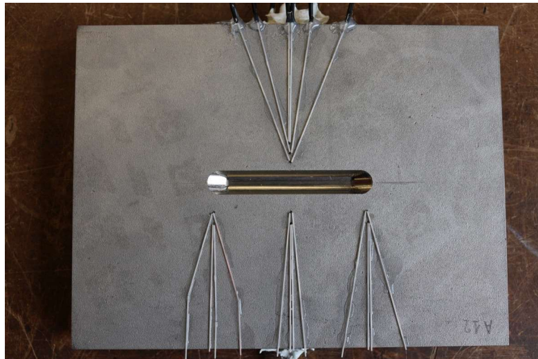
Fig. 3 TG6 specimen prior to welding, showing machined slot and top surface thermocouples
