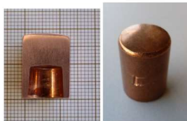
Fig. 1 Reference electrodes type A0-13-18-32 – diameter 13mm, curvature radius 32mm
