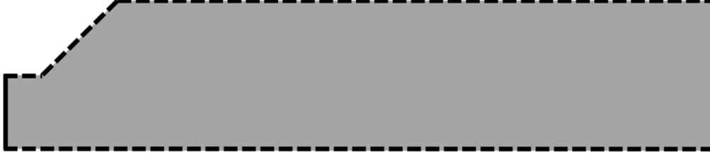
Fig. 2 Boundary conditions used in the simulation (during the first pass of two pass weld). The dashed line represents convection and radiation and the solid line seen on the left of the figure represents a symmetry boundary condition.
