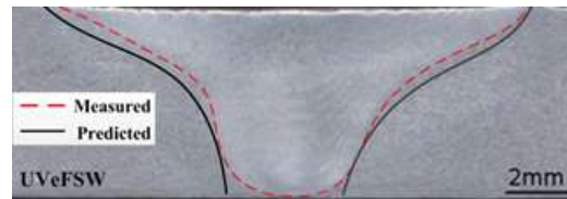
Fig. 12 Comparison of the calculated and measured TMAZ profile in UVeFSW
