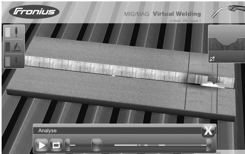
Fig. 11 Screenshot of the analysis module as implemented in the Fronius Virtual Welding® training system
