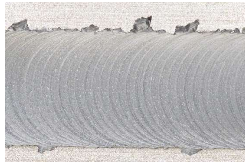
Fig. 3 Banded structure of a friction stir weld
