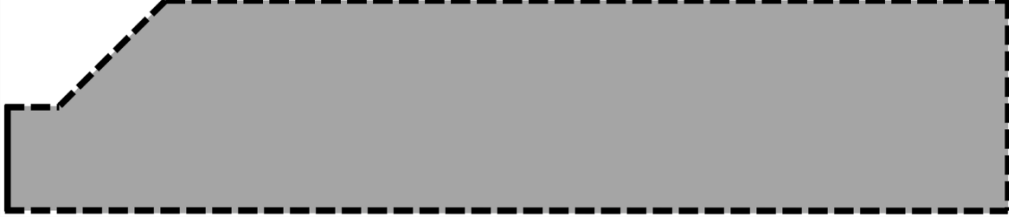
Fig. 2 Boundary conditions used in the simulation (during the first pass of two pass weld). The dashed line represents convection and radiation and the solid line seen on the left of the figure represents a symmetry boundary condition.
