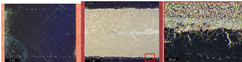
Fig. 14: Observation of a part of the welding surface of the PVR specimen F: before chemical attack (left) and after electrolytic etching (center and right).
