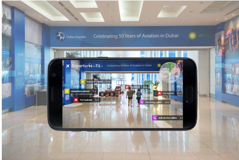
Fig. 2. Concept design for a prototype location-based AR asset management app in an airport for utility managers
