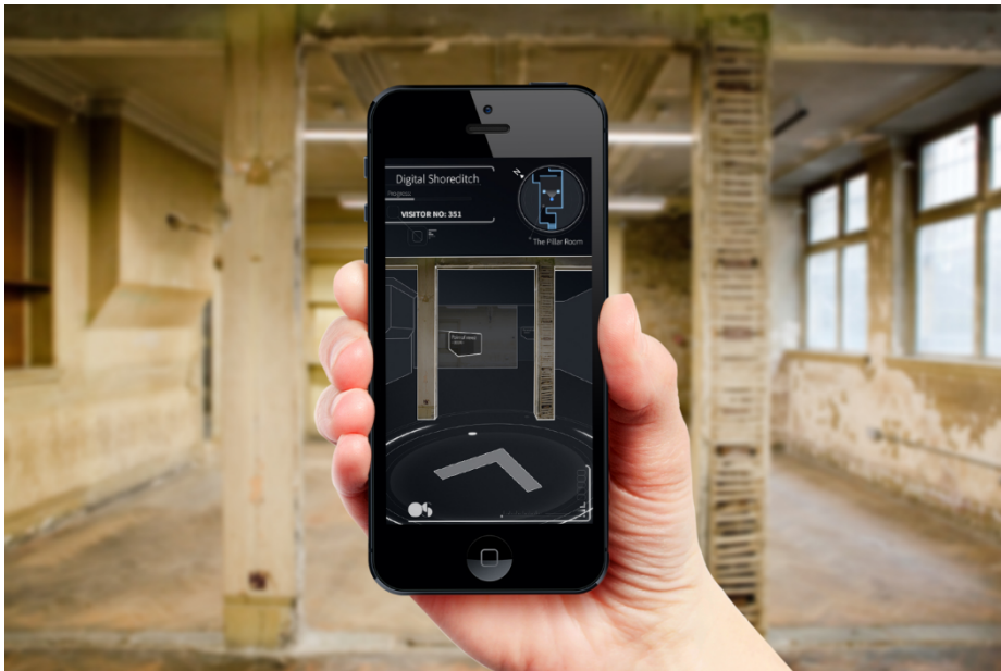
Fig. 7. Concept design of a location-based AR app used indoors to reveal the 'beyond the wall' features of the building that the human eye can not normally see. The positional accuracy of 2-3 meters is achieved by using over 30 iBeacons installed in the underground of Shoreditch Town-hall basement
