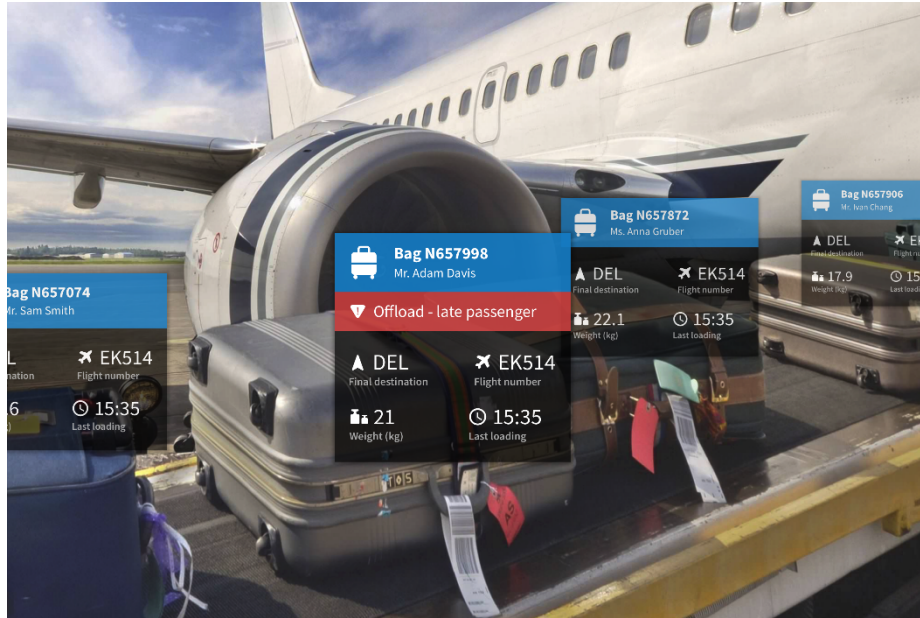
Fig. 4. AR dashboard for the baggage handler staff connected to an autonomous baggage handling system
