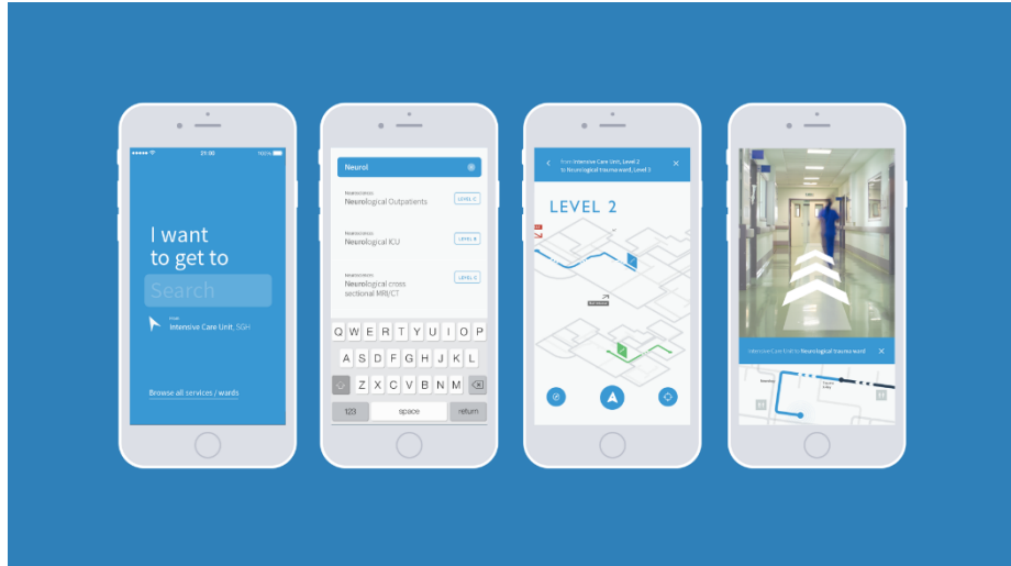
Fig. 1. UI prototype of an indoor navigation app powered by iBeacons for patients, visitors and staff
