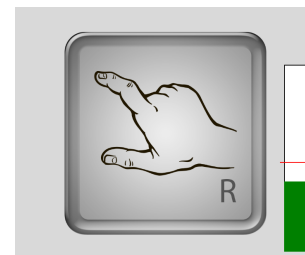
Figure 2: Subject screen. Pictogram of a hand represents mental imagery task cue and bar on the right side shows real-time RMS of subject's EMG from forearm muscles.
