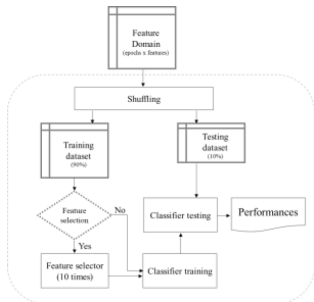
Figure 1: Validation approach. For each iteration (10 in total) the steps in the hatch block were repeated. Specifically, feature domain was shuffled and divided in training and testing dataset. The former was used to train the classifier (and to select the best two or ten features, if that was the condition under investigation), the latter to test the classifier. The performance index was computed for each iteration.
