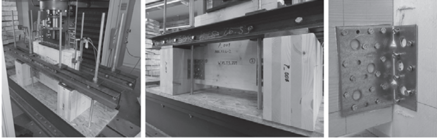
Figure 5.10: test configuration applied for shear loaded angle brackets in a wall-to-floor joint (internal designation W_V1_T3 )
