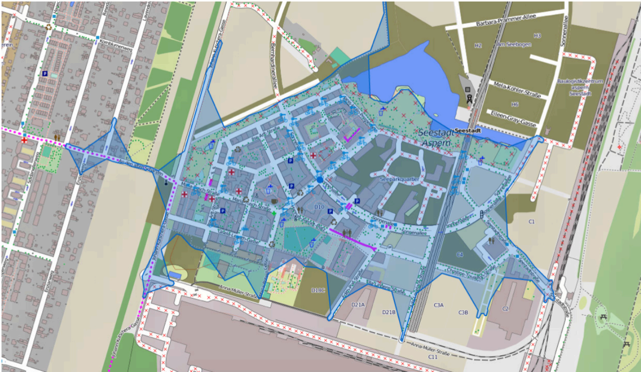
Fig. 52: Example of GIS Isochone Map of Parking Garages in Seestadt Aspern Vienna
