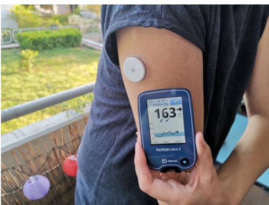
Fig. 24: Freestyle Libre sensor and reading device displaying tissue glucose of the past eight hours. Source: SW
