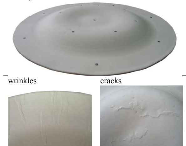
Figure 11: Optimised demonstrator model and failure criteria
