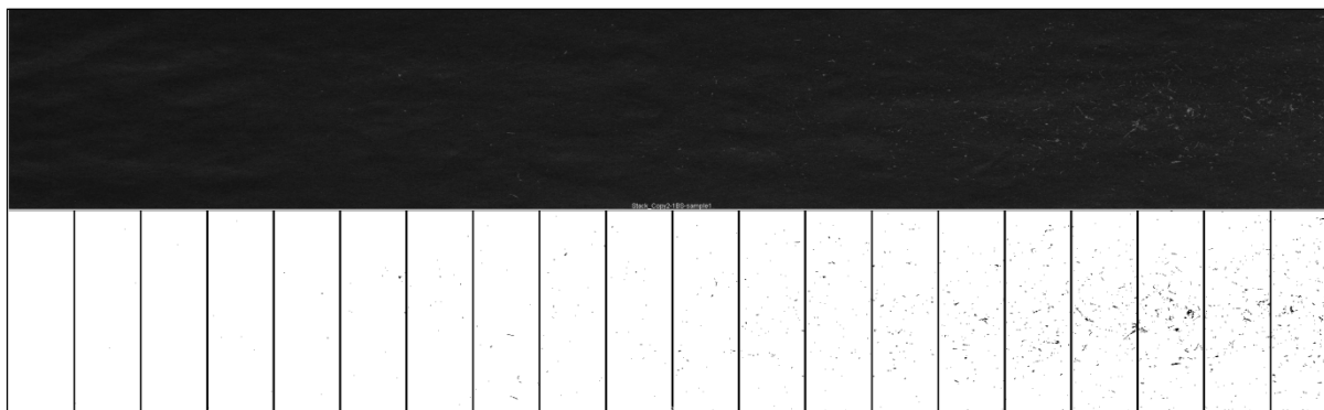
Figure 1. Example of montage obtained with ImageJ, including the original scanned image of the printed strip and the processed image. Quantification of lint particles removed from the printed strip was carried out in 20 adjacent segments, each corresponding to a different/increasing printing speed.
