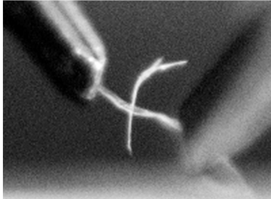
Figure 3. Side-View: An IPFB grasped with microgrippers standing as a vertical cross.
