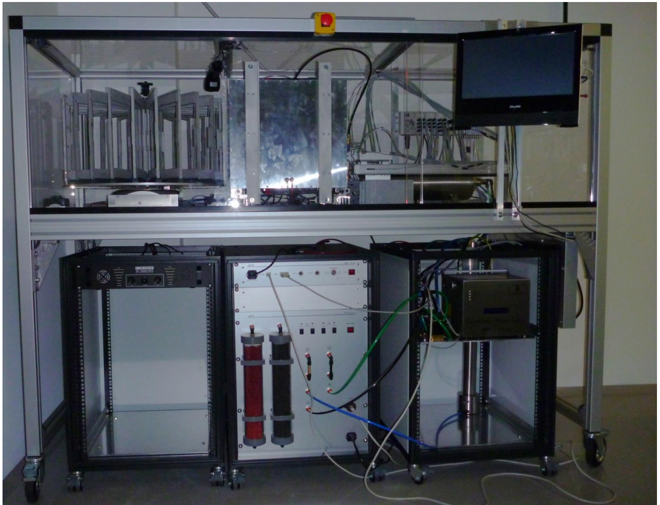
Figure 2. Complete ADT measurement device from left-to-right, top-to-bottom: carousel slide tray, measurement chamber with built-in loudspeakers, cylindrical sampling unit, flow control unit with gas purification and particle analyser.
