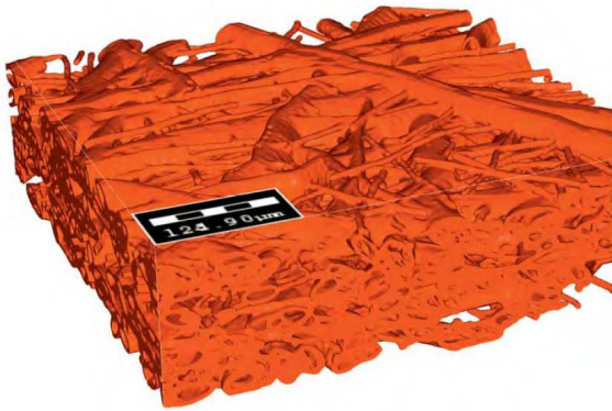
Figure 1: Stochastic realization of the micro-structure of a CTMP lab sheet in PaperGeo.
