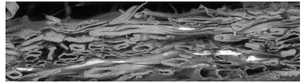
Figure 2: SEM micrographs of CTMP performed at Albany International.
