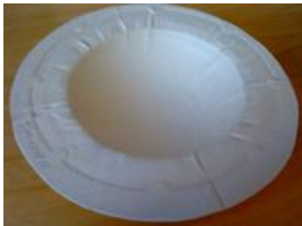
Figure 7: Paperboard from mechanical pulp (HT-CTMP) formed in the deep mould (12 % nominal strain)
