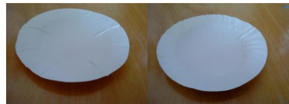
Figure 5. Two types of wrinkles: formed dry (left) and formed with significant amounts on water on upper surface (right)
