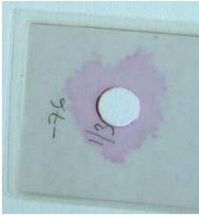
Figure 4: A sample from the pressurized edge wick experiments.
