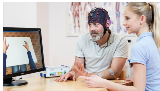
Figure 6. The experimental setup with avatar feedback and FES.
