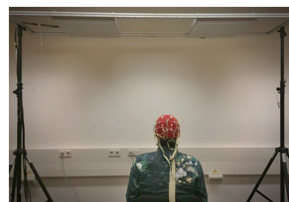
Figure 3: The experimental setup. The picture depicts a participant wearing an EEG cap and the LED panels.
