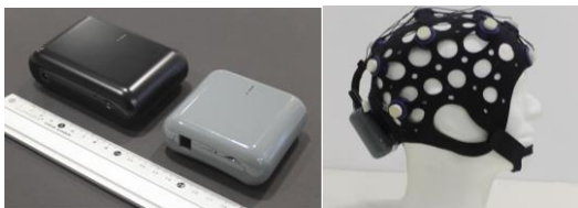
Figure 1: 32- and 16-channel MoreGrasp amplifiers (left). 16-channel system with the sensors and amplifier on a commercial cap (right).
