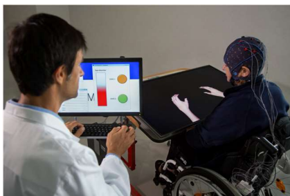
Figure 1: Training session with the Promotær. The patient is seated on a wheelchair with arms resting on a pillow. A visual representation of the forearms and hands is given on a dedicated screen, resembling the patient's own hands. The patient is asked to perform MI of affected hand and the therapist is provided with continuous feedback of the patient's EEG and EMG activity (recorded from forearm muscles).
