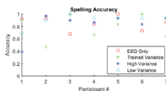
Figure 1. This figure shows the spelling accuracy given the four different configurations of the Bayesian update classifier.
