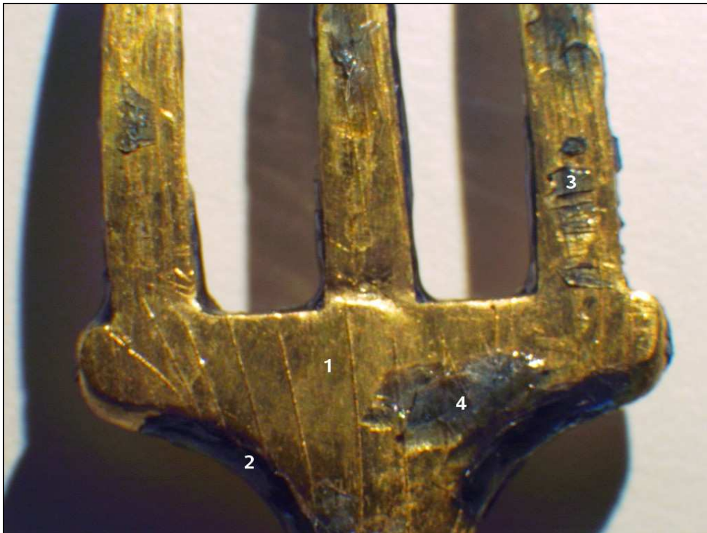
Figure 2. Trident of the Poseidon figure from the Saliera. The numbers indicate the positions for analysis (1 – gold body, 2-4 – enamel).
