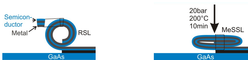
Figure1. Formation of RSL by rolling up and MeSSL by subsequent pressing
